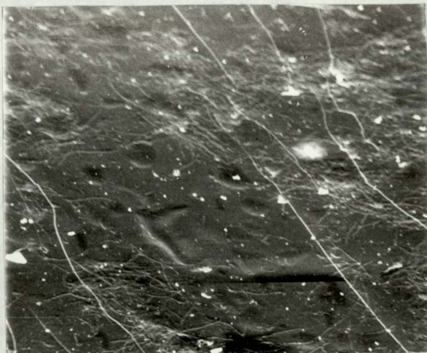
PHOTOGRAPH 15 Surface of Cuprophane (X1000)
