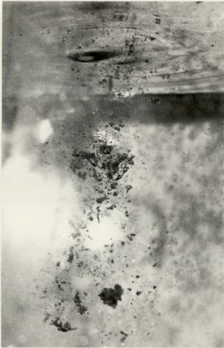
Plate XII Short exposure photograph of a tin drop showing complete fragmentation.
