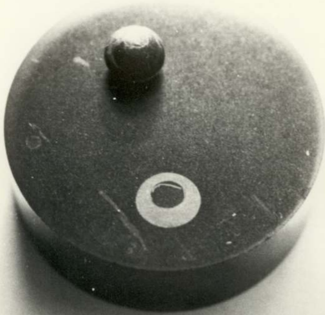
Plate IV Solid sphere of copper together with a similar sphere in cross-section.
