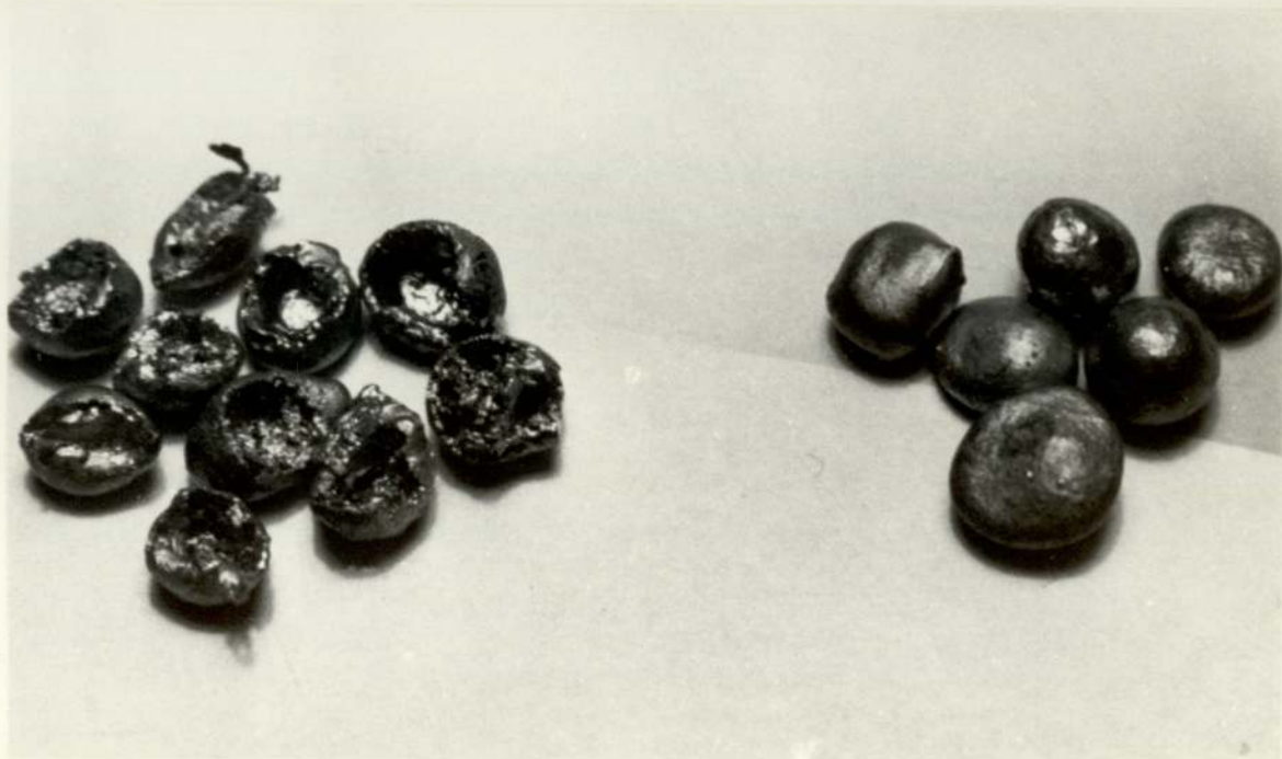
Plate V Partially fragmented copper drops together with some showing no signs of fragmentation.
