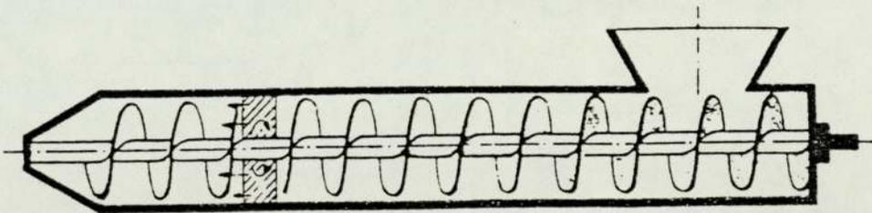
Fig 5.1 Extruder - single or twin screw
