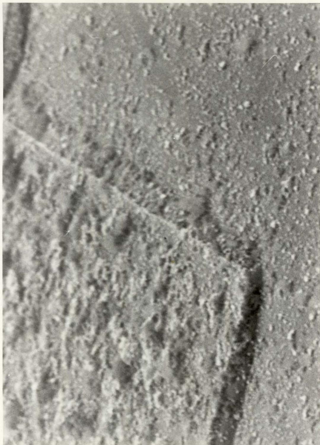
Fig.31. Si etched in  $\text{CCl}_4$  plasma.
