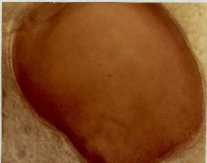
Plate 17 (PE + 20%PVC) Sample during 330 hours heating time at 100^{\circ}\text{C} , M_n=100
