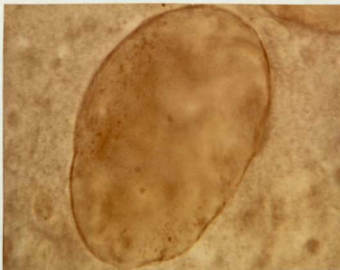
Plate 16 (PE + 20%PVC) Sample during 150 hours heating time at 100^{\circ}\text{C} , M_n=100
