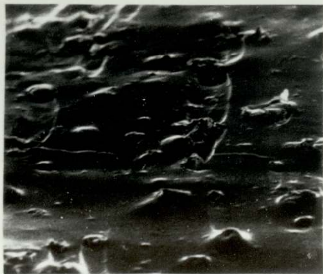
Plate 10 (PE + 20% PVC)X1000 (S.E.M)
