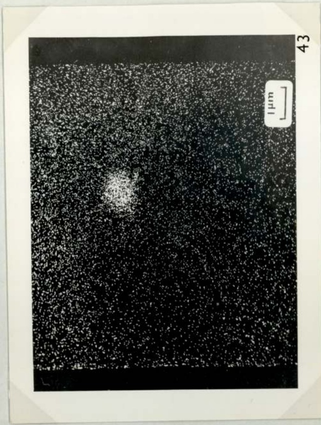
Figure 43: The M_{\alpha\beta} x-ray image of the area shown in Figure 42.
