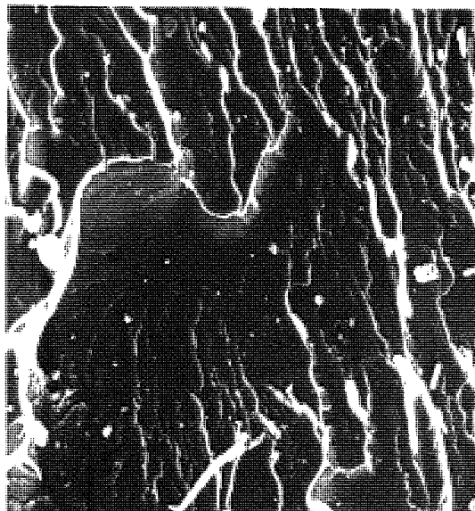
PLATE 5.9 THE TWO FRACTURE TYPES TYPICAL OF 'C5' GEL COPOLYMER SEM X65
