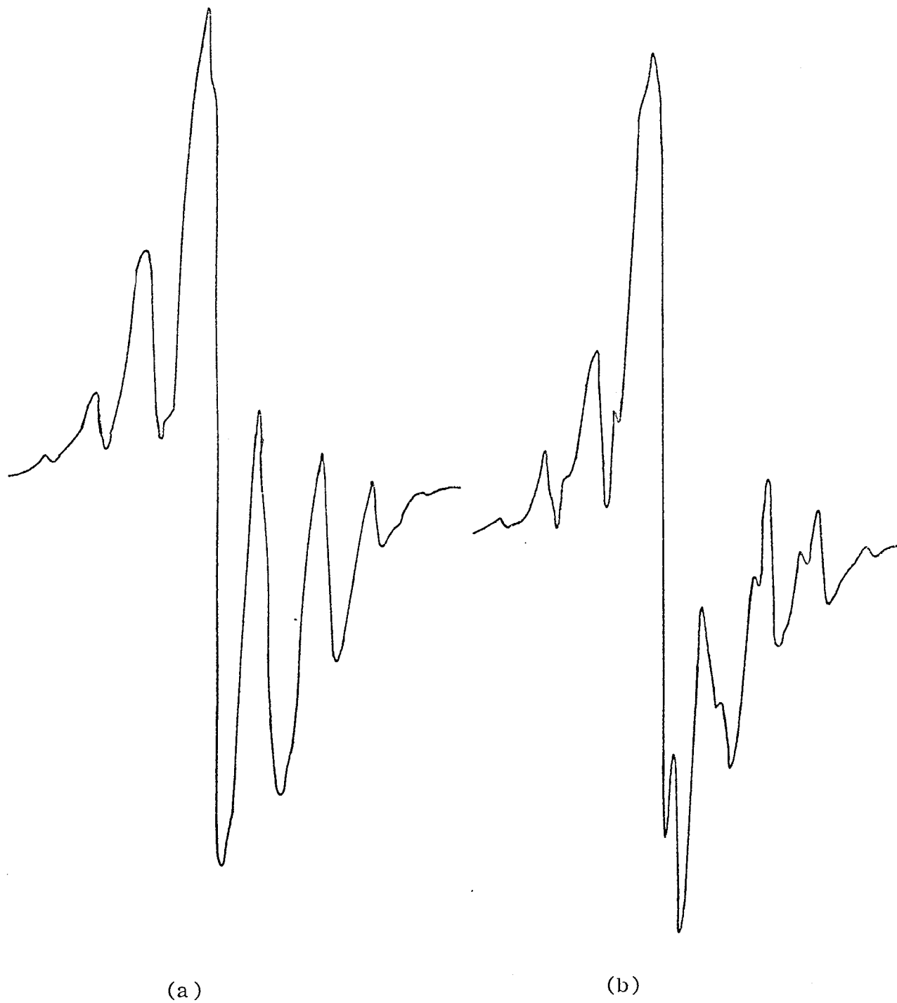
Fig 4.18 Change of E.S.R. spectrum during radical decay of \gamma -irradiated polypropylene in vacuo at 55°C.
