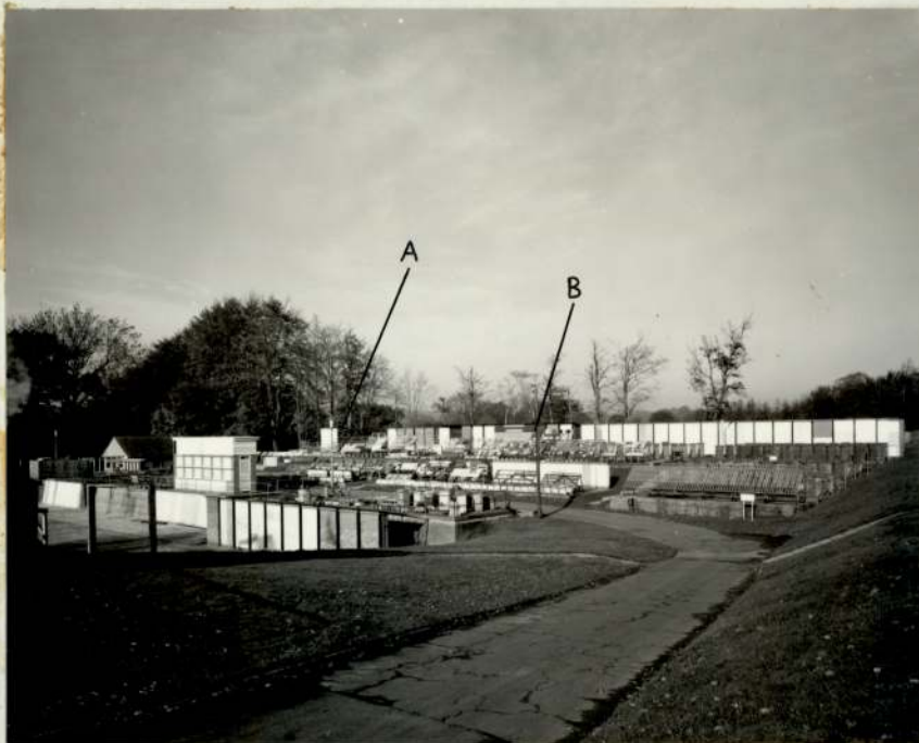
PLATE 1 - View of the Building Research Station exposure site, showing (A) exact location of sample rack in relation to (B) the solar radiation detectors.
