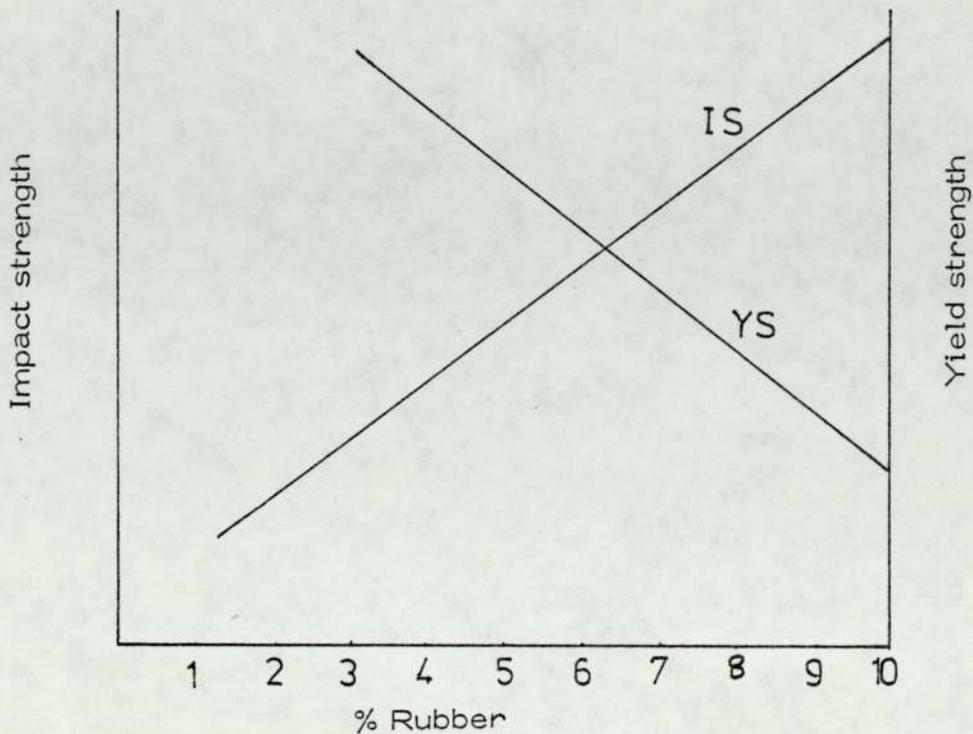
Figure 6. Effect of co-polymerisation of acrylonitrile on the properties of PS/PBD systems.
