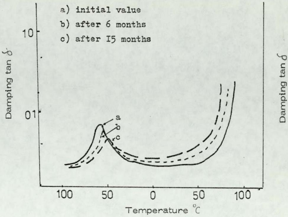
Figure I7. Dependence of mechanical damping  $\tan \delta$  on the temperature (T) for ASA.
