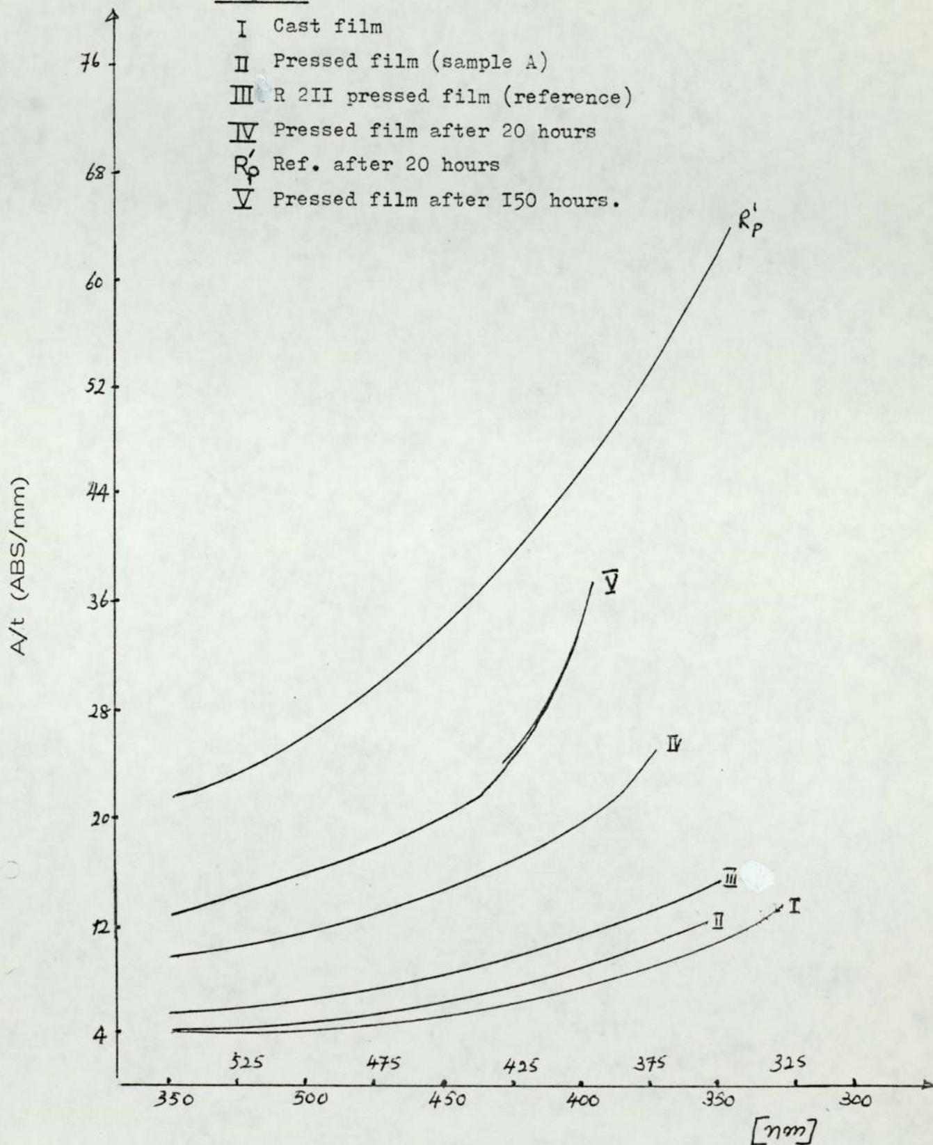
Figure 57. Development of visible spectrum on uv ageing of ABS films using Xenotest I200.
