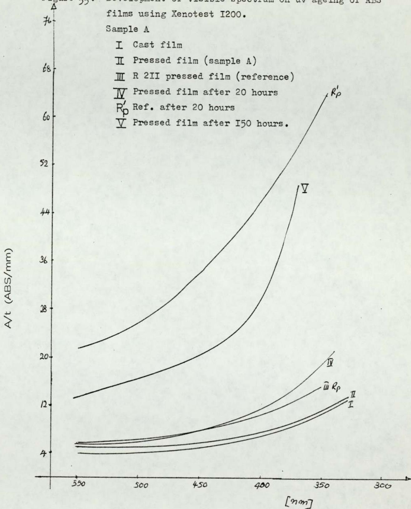
Figure 56. Development of visible spectrum on uv ageing of ABS films using Xenotest I200.
