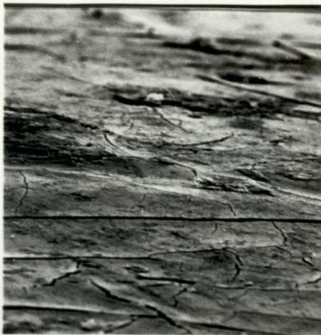
Photograph 6.3. The scanning electron micrograph of a paint sample containing vermillion.
