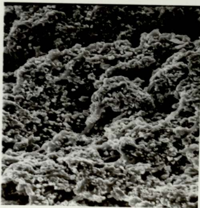
Photograph 6.4. The scanning electron micrograph of a paint sample containing vermillion
