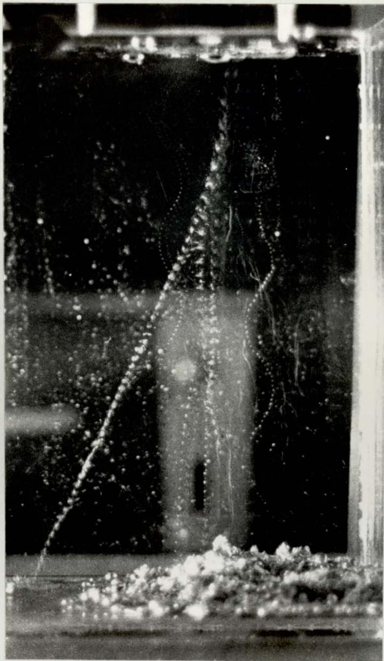
FIGURE 33a. Molten tin drops at  $300^{\circ}\text{C}$  falling from a height of 23 cm into distilled water at  $20^{\circ}\text{C}$ . The drops were photographed in a stroboscopic light at 9500 flashes per minute.
