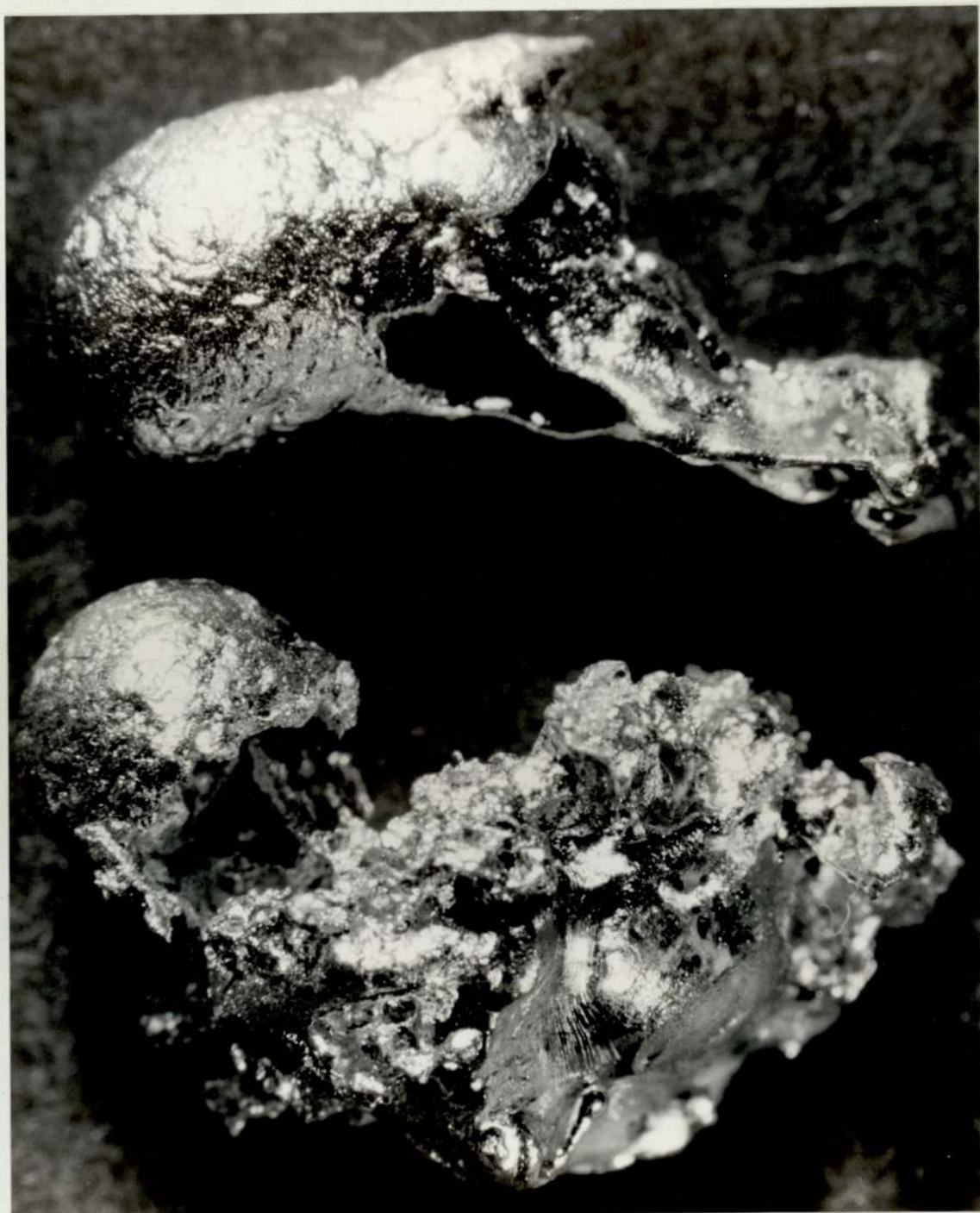
FIGURE 39. Partially Disintegrated Tin Drops
