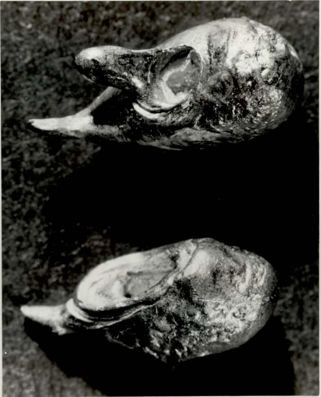
FIGURE 47. Lead drops showing hole formation near to their centre of gravity and also the hollow crust.
