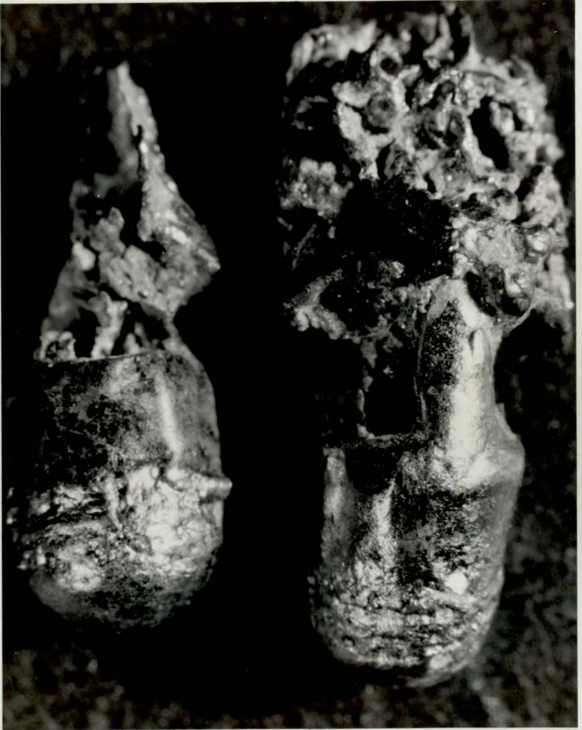
FIGURE 40. Partially Disintegrated Lead Drops
