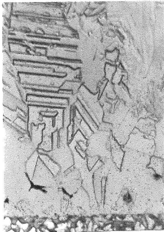
Fig. 8.2. Electrodeposited copper, transverse section etched in ferric chloride reagent. x 150, enlarged x 3.
