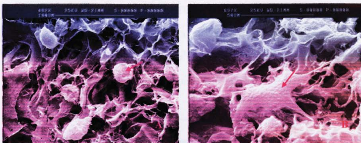
Figure 20: SEM of NHEK growth on 1:8 w/w collagen:PCL biocomposites for 1 (A) and 3 (B) days. (Arrow indicates the cell body.)
