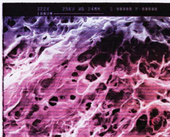
Figure 12: SEM of 1:8 w/w collagen:PCL biocomposites before (A) and after incubation in PBS at 37°C for 3 (B) and 7 (C) days.
