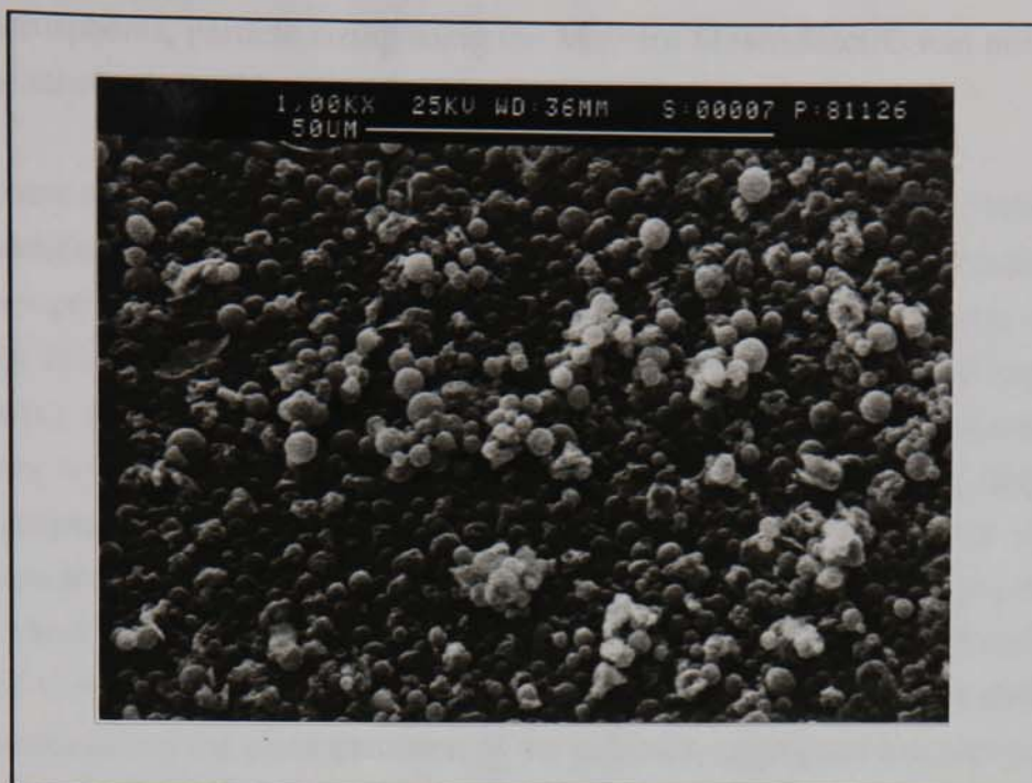
Figure 8.2. Scanning electron micrograph of BSA microspheres prepared by spray drying
