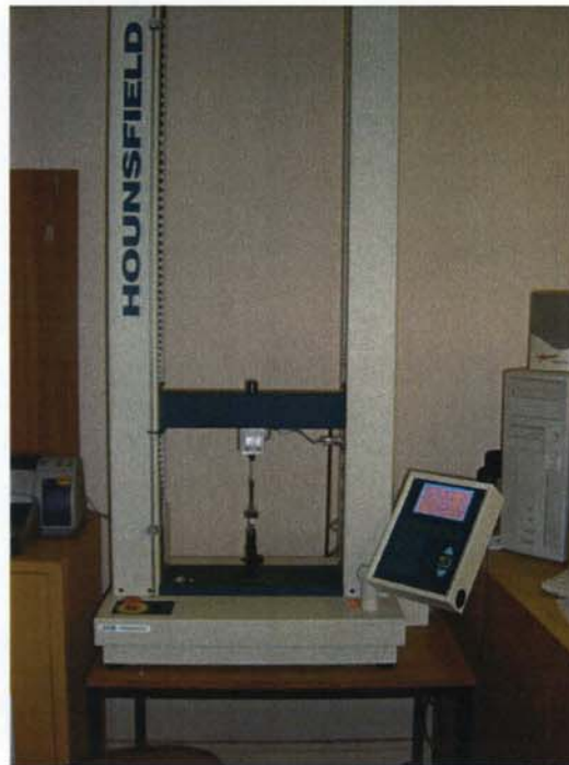
Figure 7.8 The Hounsfield S Series Universal Testing Machine
