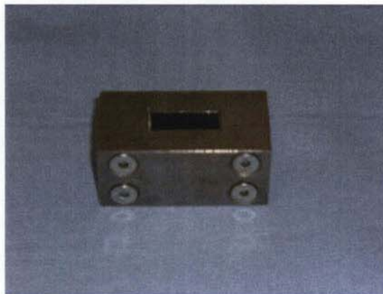
Figure 7.6 Roberts 20 x 7 mm four piece stainless steel die held together with screws.
