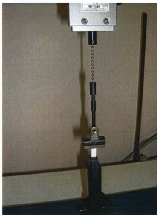
Figure 7.9 Avicel PH105 wafer held between upper and lower clamps for elongation
