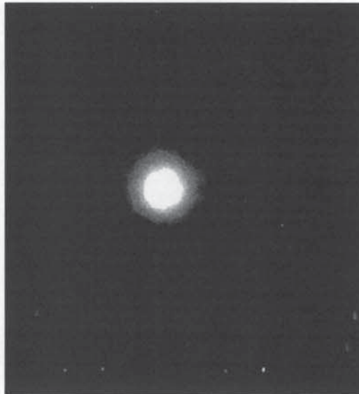
Figure 7.27 X-ray image of ibuprofen compact of negative porosity, the white dots indicate preferred orientation
