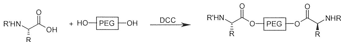
Figure 9.3 Direct esterification of PEG with amino acids
