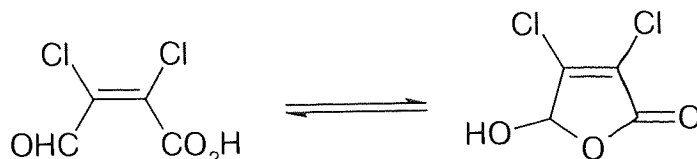
Scheme 6.1.1: The two forms of mucochloric acid.
