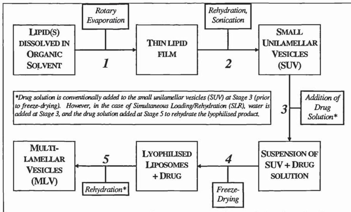
FIGURE 2.9: Flow diagram showing the main stages of the DRV process
