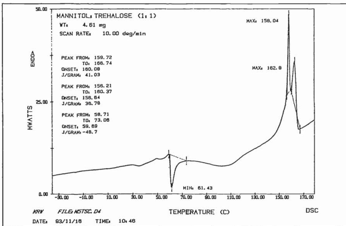
FIGURE 3.3: DSC reheating profile of a 1:1 (w/w) mixture of mannitol and trehalose
