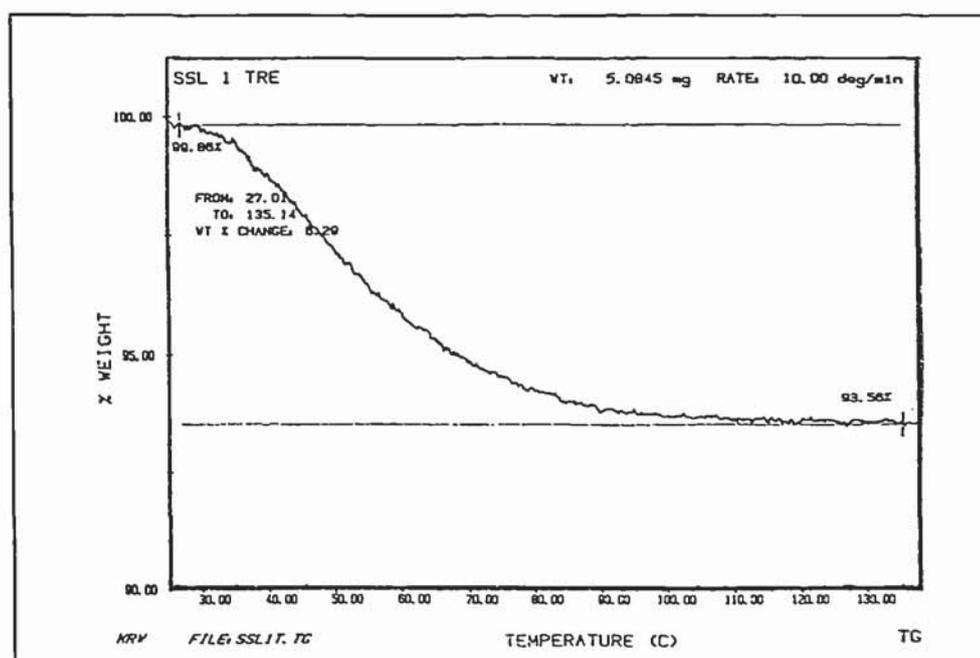
FIGURE 2.4: Typical TGA weight loss profile for a lyophilised product
