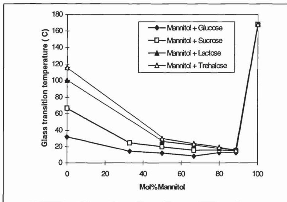
FIGURE 3.5: Graph showing relationship between proportion of mannitol in mixture and glass transition temperature
