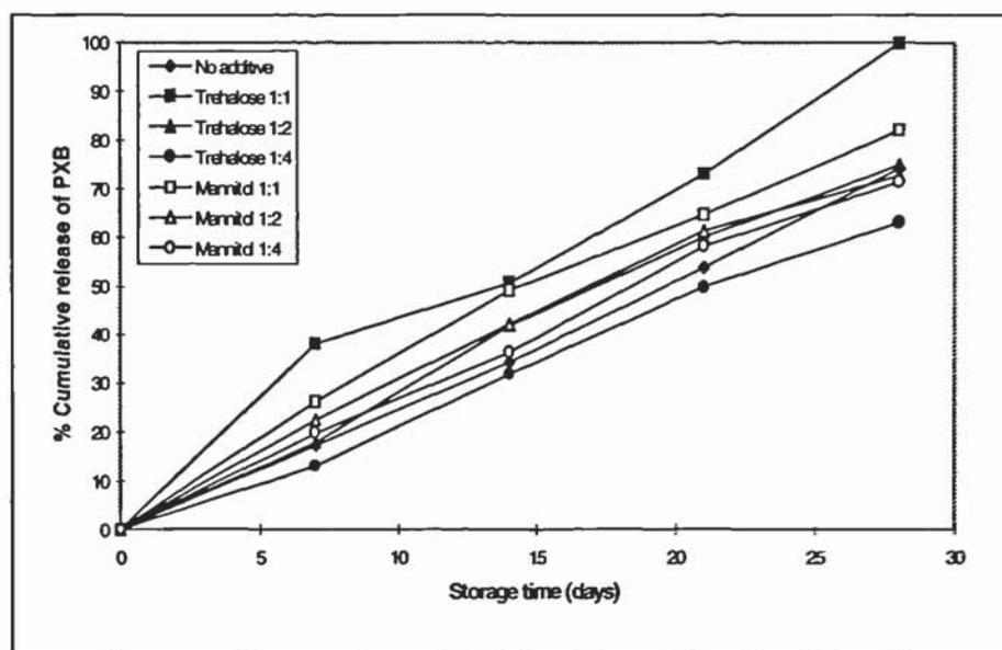
FIGURE 5.6: Leakage of PXB from liposomes into aqueous medium during storage at 4°C
