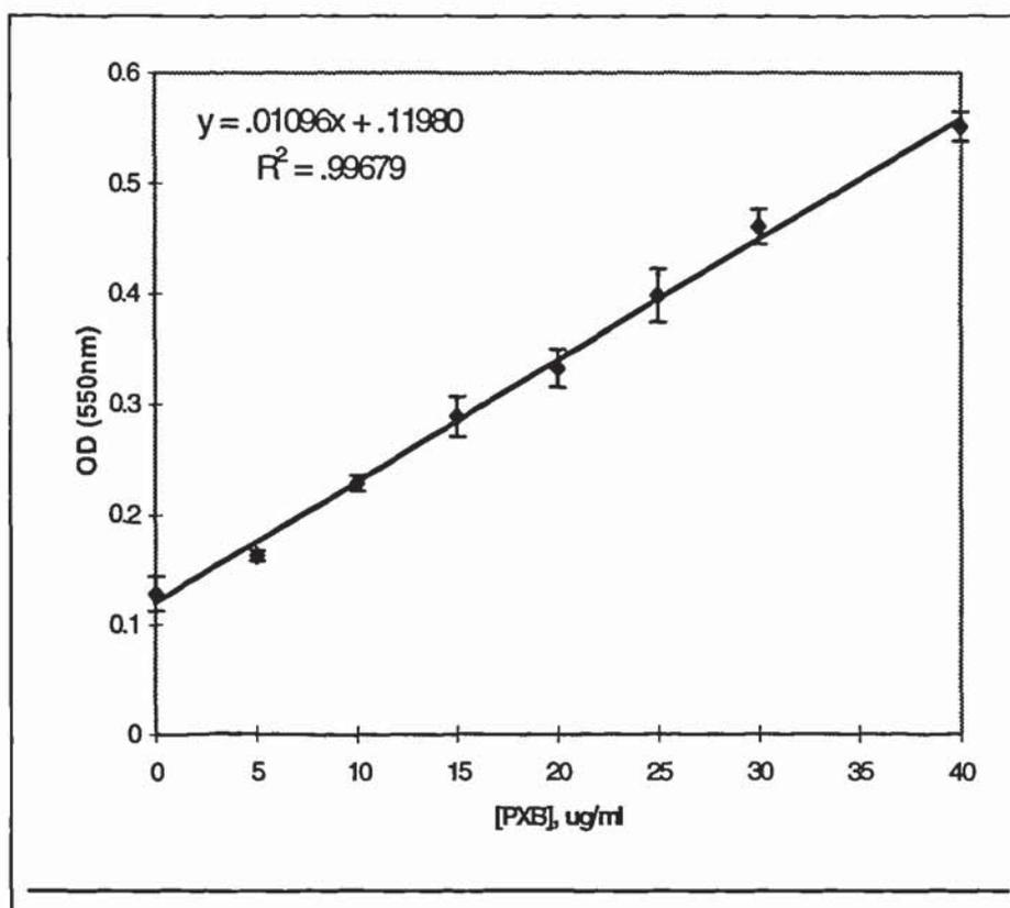
**FIGURE 2.7:** Typical calibration plot for PXB standard solutions analysed by microassay
