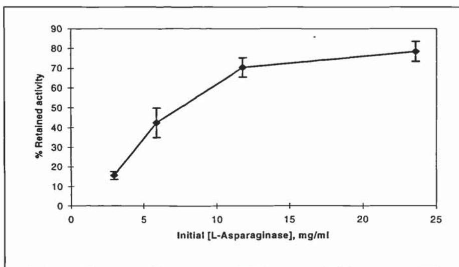
**FIGURE 4.10:** Graph to demonstrate the relationship between initial protein concentration and retained biological activity following freeze-drying, determined using the AHA assay developed from Frohwein et al. (1971)
