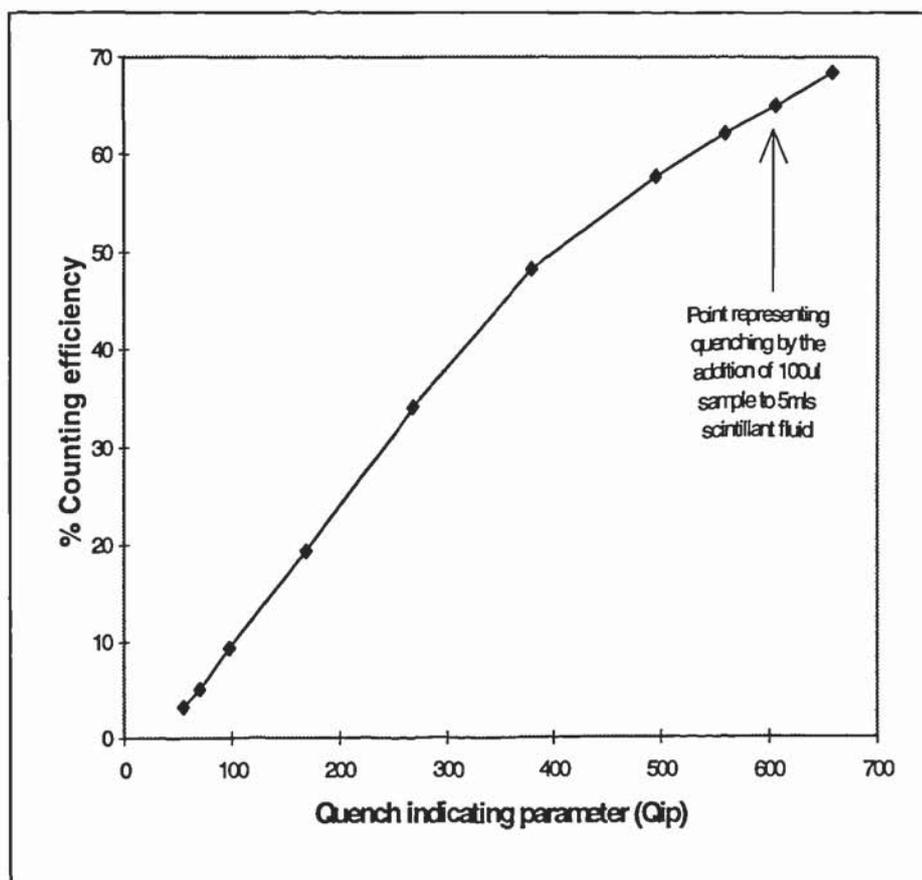
FIGURE 2.11: Quench curve for  $^3\text{H}$ -PXB standards diluted in Optiphase Hi-Safe 3 scintillant fluid (5ml)
