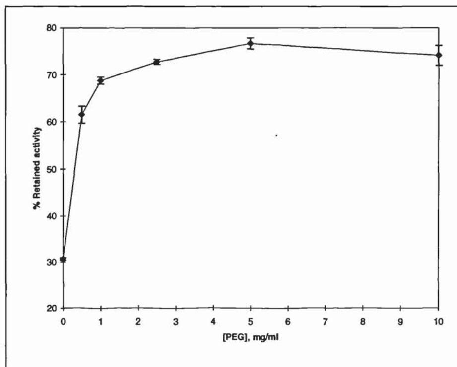
**FIGURE 4.8:** Effect of PEG concentration on the retention of enzyme activity of *L*-asparaginase immediately following freeze-drying, as determined using the AHA assay developed from Frohwein *et al.* (1971).
