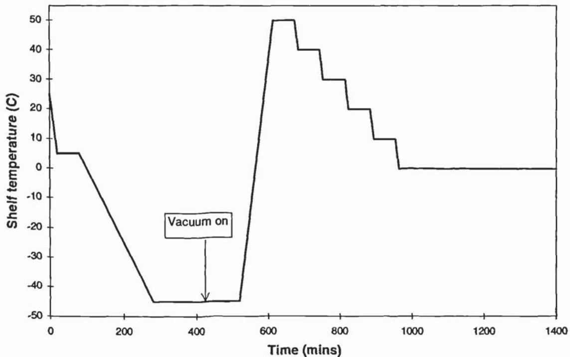
*FIGURE 6.2: Flow diagram representing the revised cycle for the lyophilisation of potassium chloride solution*
