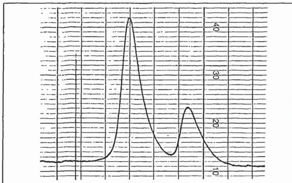
**FIGURE 2.5:** Profile showing tetramer and monomer peaks for a solution of lyophilised and reconstituted *L*-asparaginase eluted from FPLC columns
