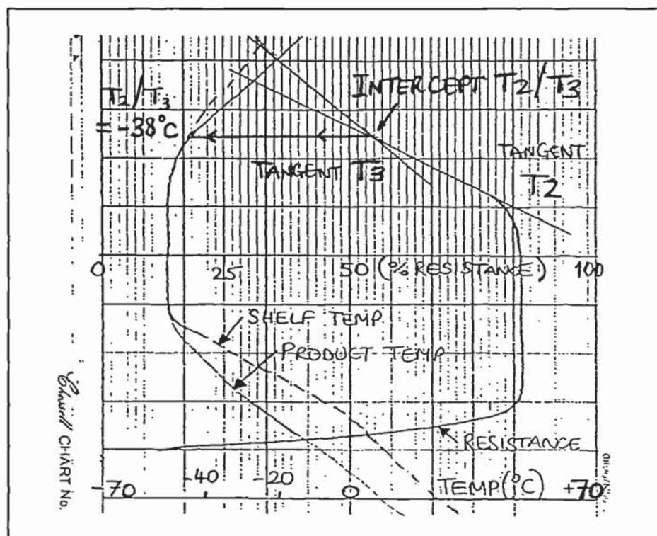
FIGURE 2.1: Typical printout from the Edwards freezing resistance analyser
