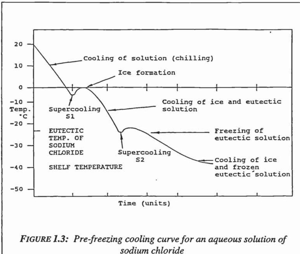
FIGURE I.3: Pre-freezing cooling curve for an aqueous solution of sodium chloride
