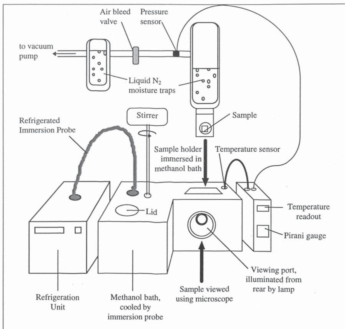
**FIGURE 2.2:** Schematic diagram of the CAMR freeze-drying microscope
