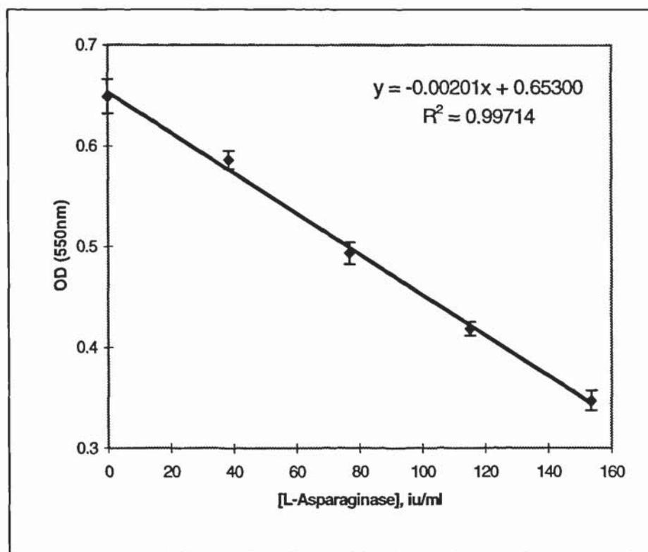
**FIGURE 2.8:** Calibration plot for L-asparaginase standard solutions analysed using the AHA assay developed from Frohwein et al. (1971)
