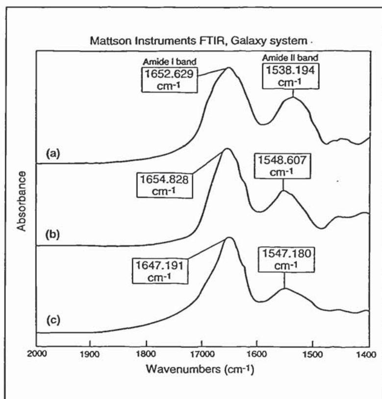
**FIGURE 4.7:** Amide band region for dried samples, as determined by FT-IR spectroscopy. Spectra shown are of L-asparaginase freeze-dried alone (a), freeze-dried in the presence of trehalose (1.0mg/ml) (b) and hydrated L-asparaginase (c). All spectra have been normalised with respect to the amide I bands.
