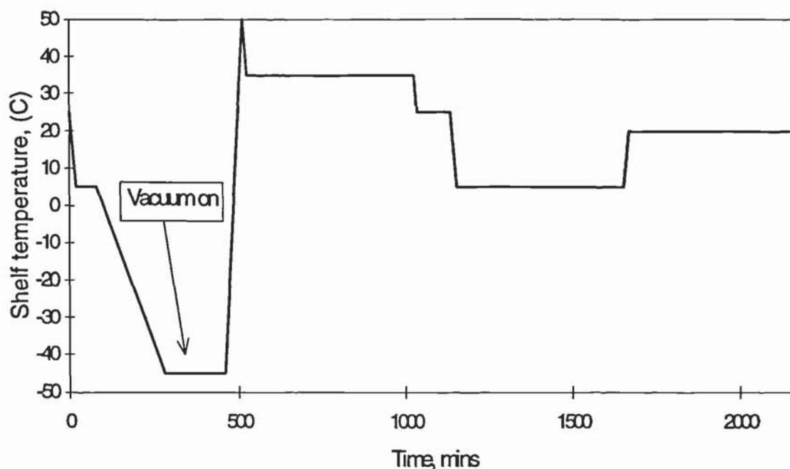
*FIGURE 6.3: Flow diagram depicting the revised freeze-drying cycle for the non-crystallising paracetamol formulation*
