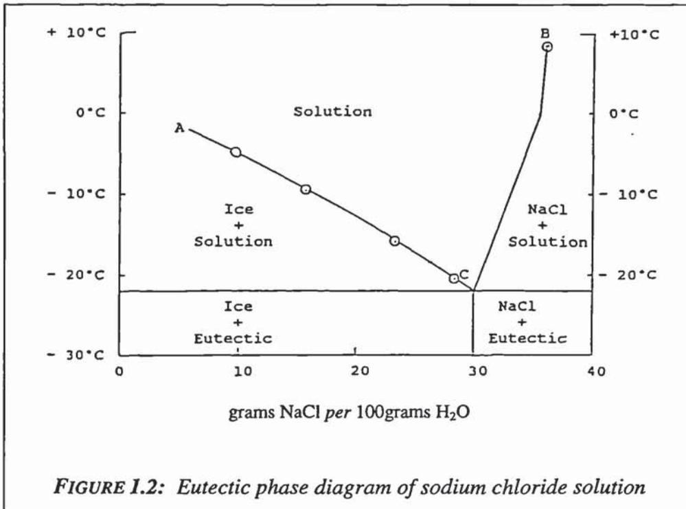
FIGURE I.2: Eutectic phase diagram of sodium chloride solution
