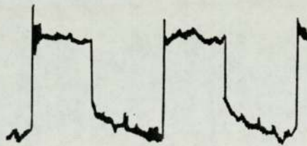
Figure 2.15 The variation of the coefficient of friction during a cycle of mild wear (after approximately 7200 cycles) The experimental conditions for both traces were:-
