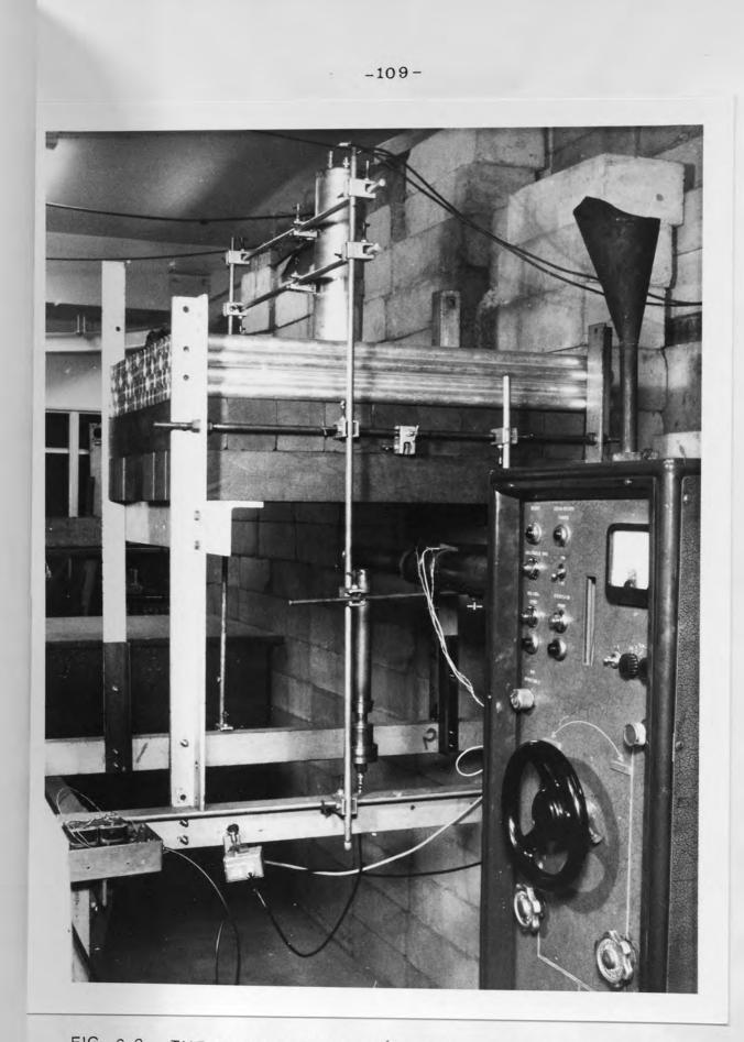
FIG. 6.3 THE SLAB ASSEMBLY (10.9 Cm. URANIUM ON TOP OF 17.8 Cm. THICK GRAPHITE), THE NEUTRON DETECTOR, THE STEEL FRAME, THE BEAM TUBE AND SAMES ACCELERATOR.
