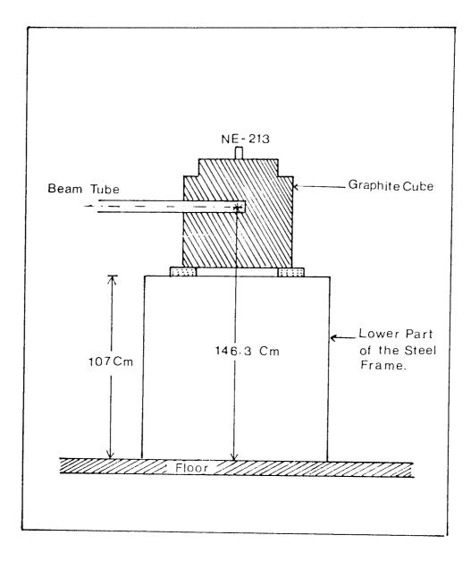
FIG. 6.2 THE STEEL FRAME (LOWER PART), GRAPHITE CUBE, THE BEAM TUBE AND THE NEUTRON DETECTOR.
