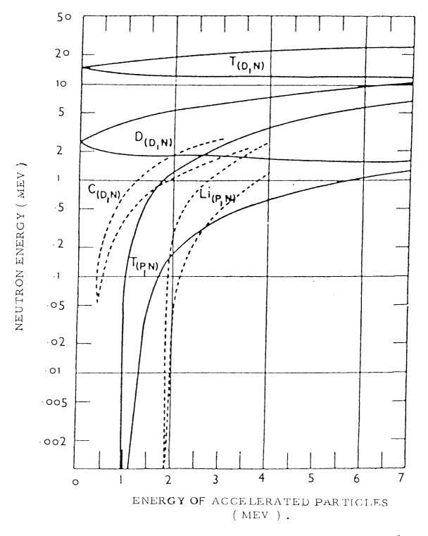
FIG. 2.1 ENERGIES OF NEUTRONS EMITTED AT  $0^{\circ}$ AND 180° FOR THE MOST IMPORTANT MONOENERG ETIC (p,n) AND (d,n) REACTIONS. (THE LOWER CURVE THE 180° ENERGY).
