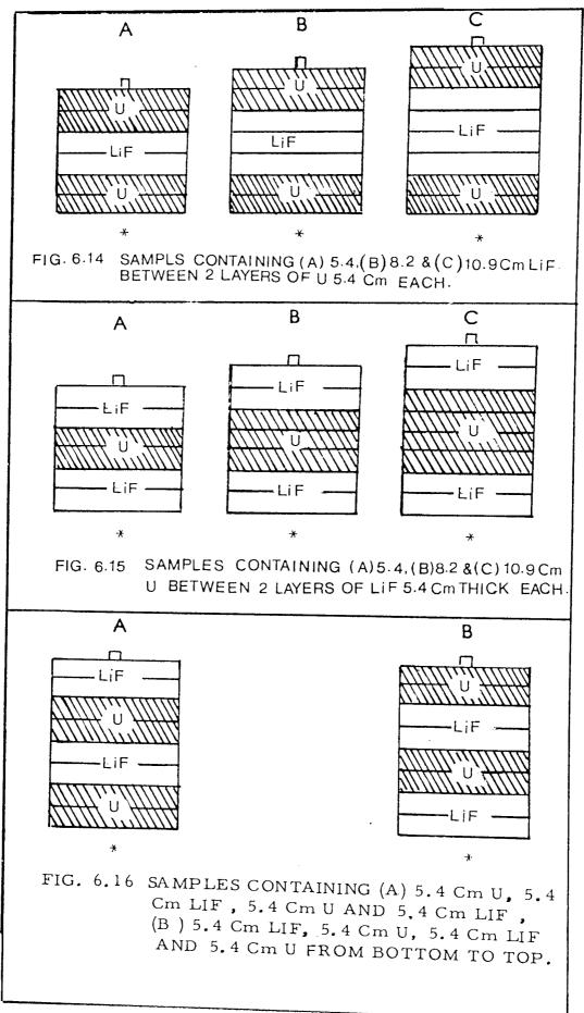
Finally, samples of multilayers of uranium and LiF were build up by putting 5.4 cm uranium on bottom followed by 5.4 cm LiF, 5.4 cm U and 5.4 cm LiF from bottom to top respectively as shown in figure (6.16 A). Interchanging LiF and uranium layers from the previous arrangement was also used as shown in figure (6.16 B).
