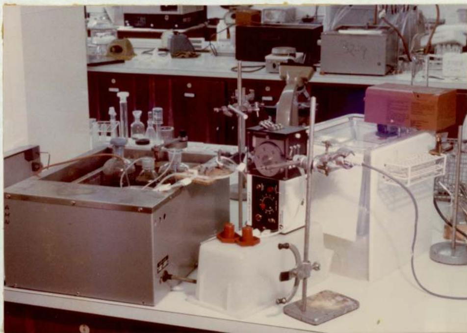
Figure 2.2. Schematic Representation of the Essential Components of the Single Cycle Perfusion System
