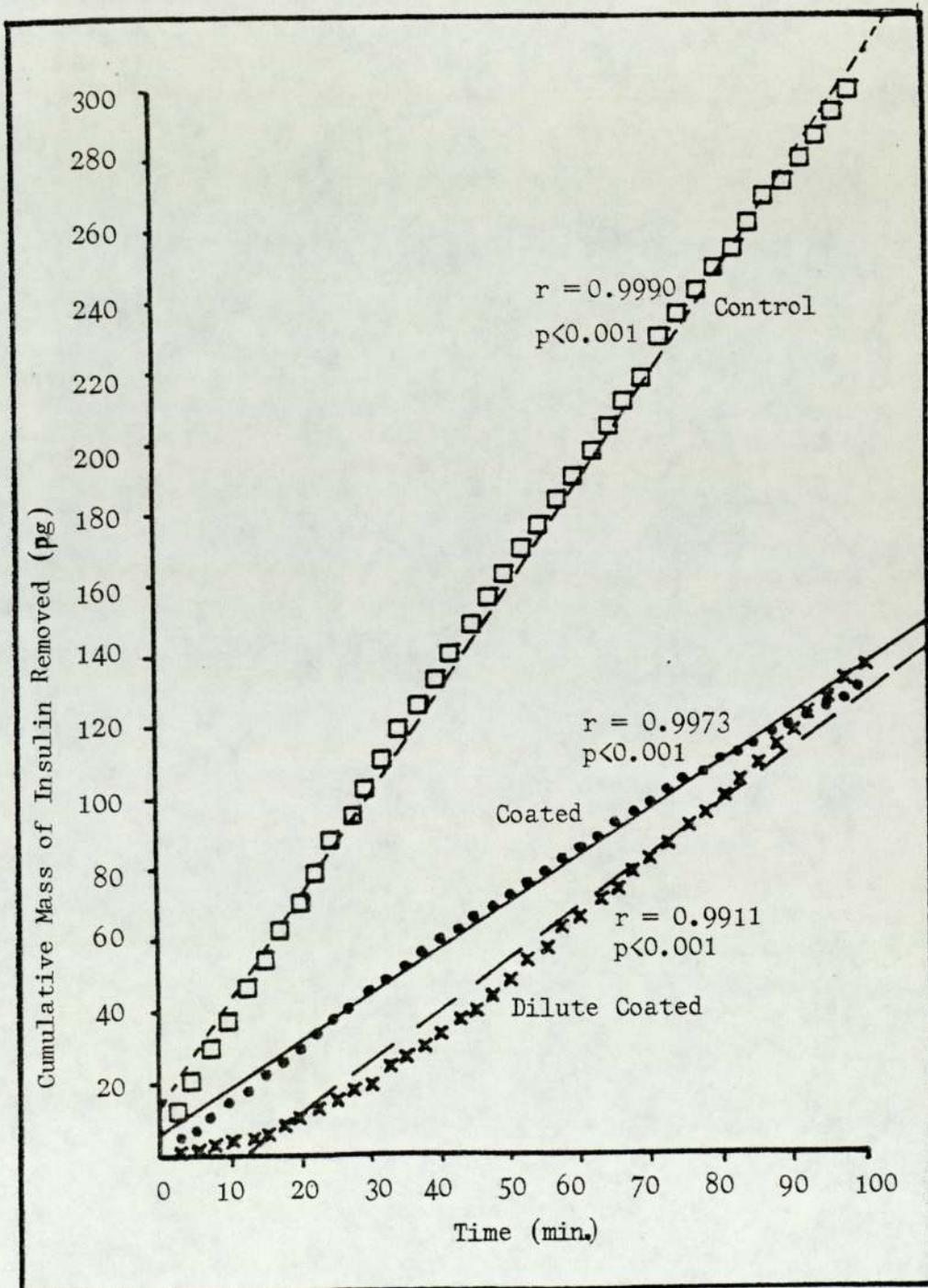
Figure 3.12. Elution of Unbound Protein from a Dilute Coated Unit with Time. Unit perfused for 100 minutes at a flow rate of 0.637 ml/min.
