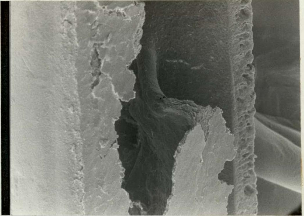
PLATE 20. Thrombus Formation in Lumen of Hollow Fibre.
