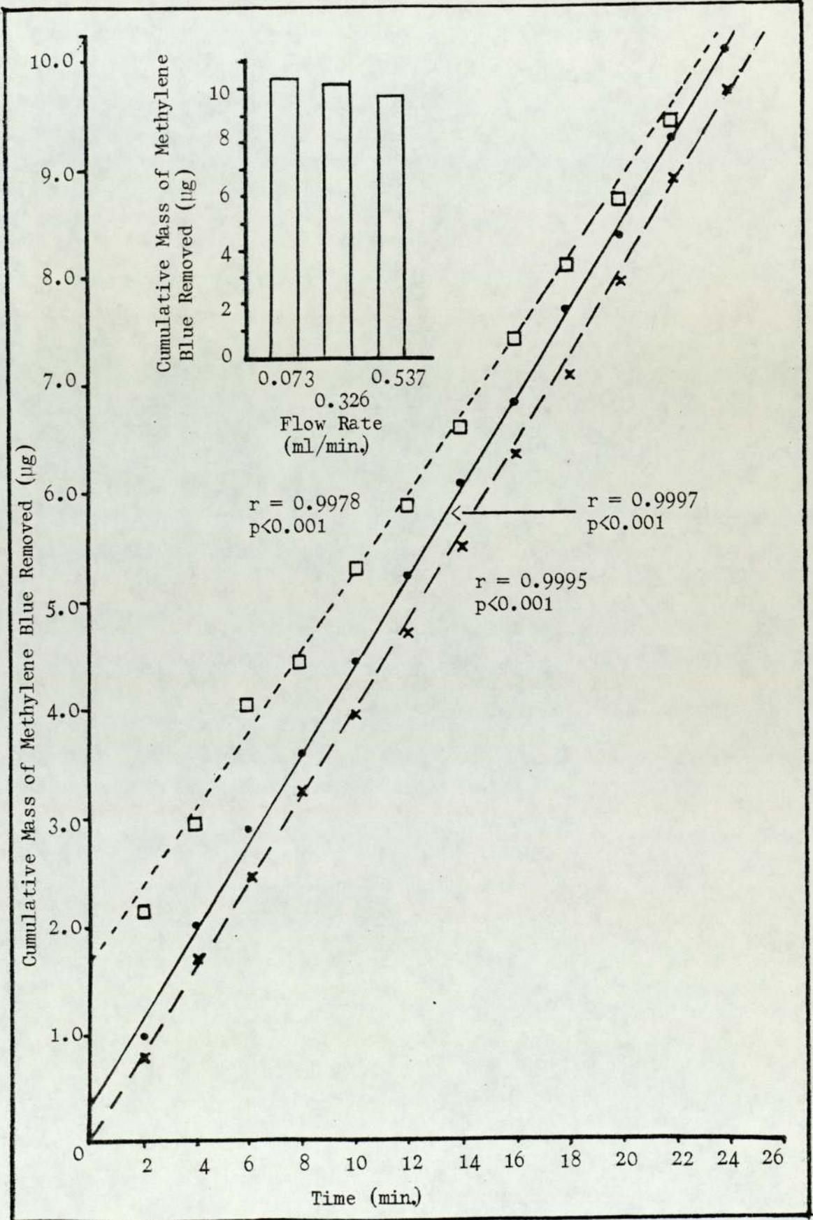
Figure 3.5. Cumulative Mass of Methylene Blue Released from Units Over a Period of 450 Minutes' Perfusion at Three Fixed Flow Rates.  $\square$  - -  $\square$  (0.073 ml/min.);  $\bullet$  - -  $\bullet$  (0.162 ml/min.); x - - - x (0.637 ml/min.). Data shown represent single determinations.
