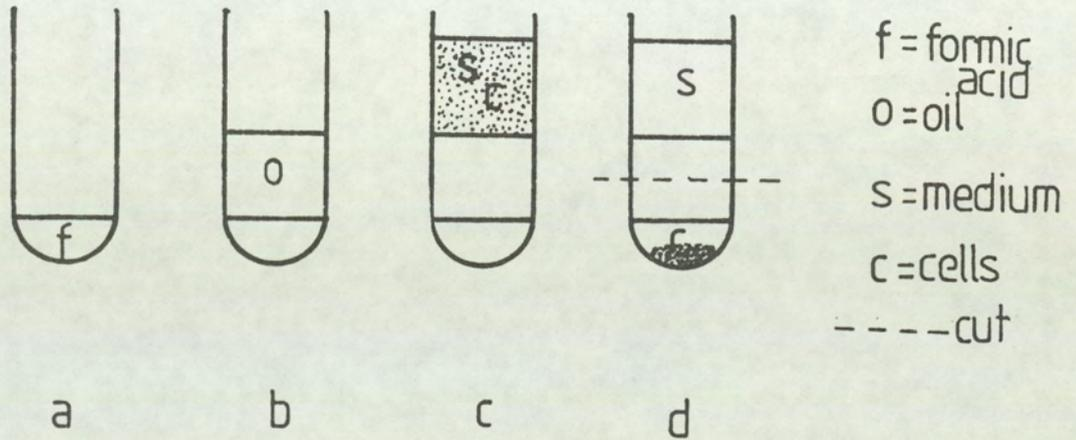
by comparing the Cr 51 remaining in the supernatant after centrifugation with that present in the cell pellet (Figure M7). This revealed that the silicone oil Ms550 proved to be superior in allowing maximum cell passage.
