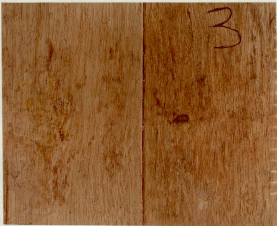
PLATE 2: stains developed on the wood veneers as a result of fungal colonisation (after exposing the wood veneers at the factory for one month).
