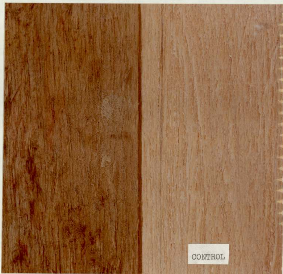
PLATE 1: ▲ - a wood veneer showing signs of severe fungal colonisation after one month exposure at the factory site - Sapele, Nigeria.
