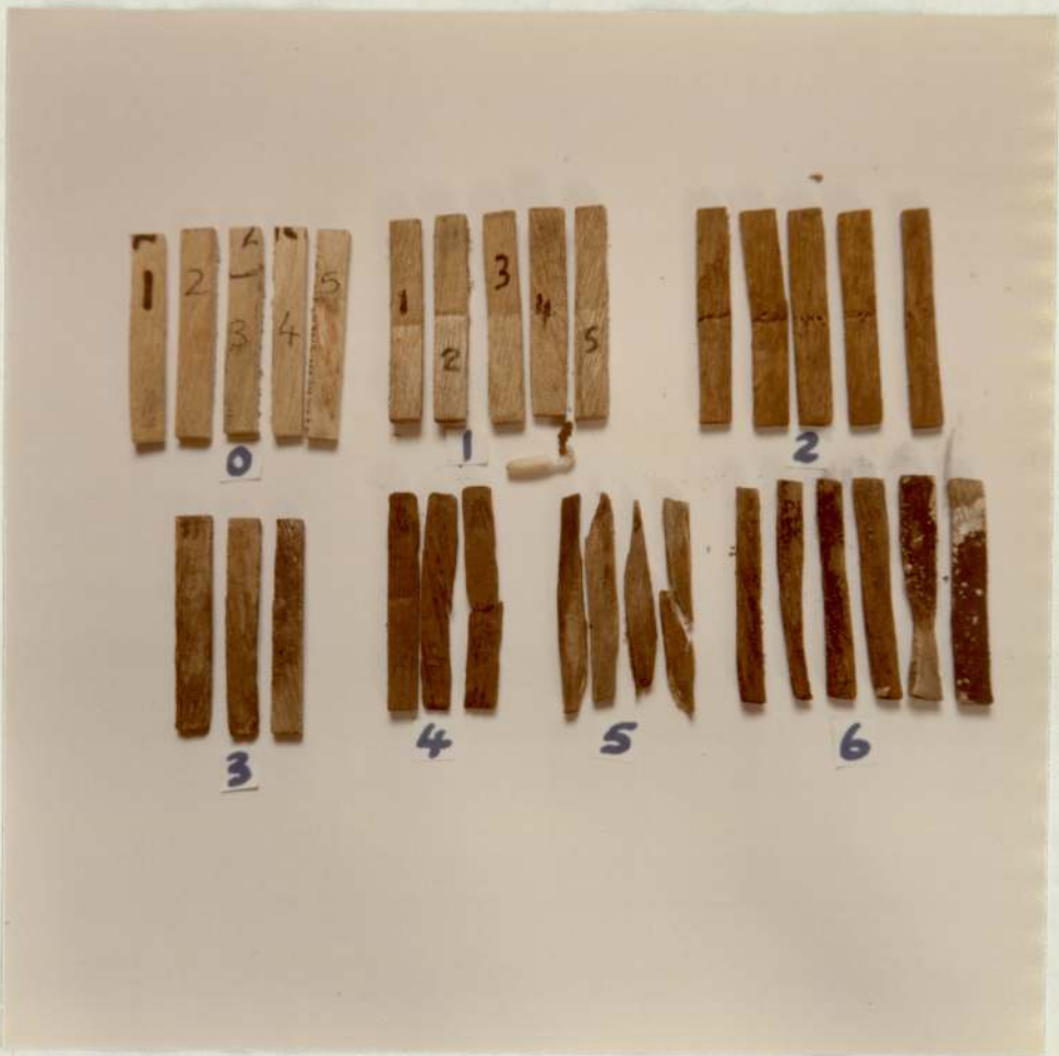
PLATE 6: shows the stages in the fungal decay of test wood pieces.
