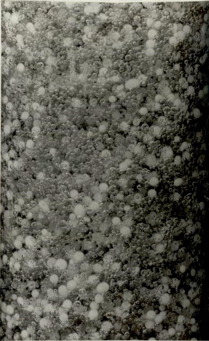
Aeration approximately 2-3 cm/sec - 8.6 cm glass column containing smooth mould pellets.
