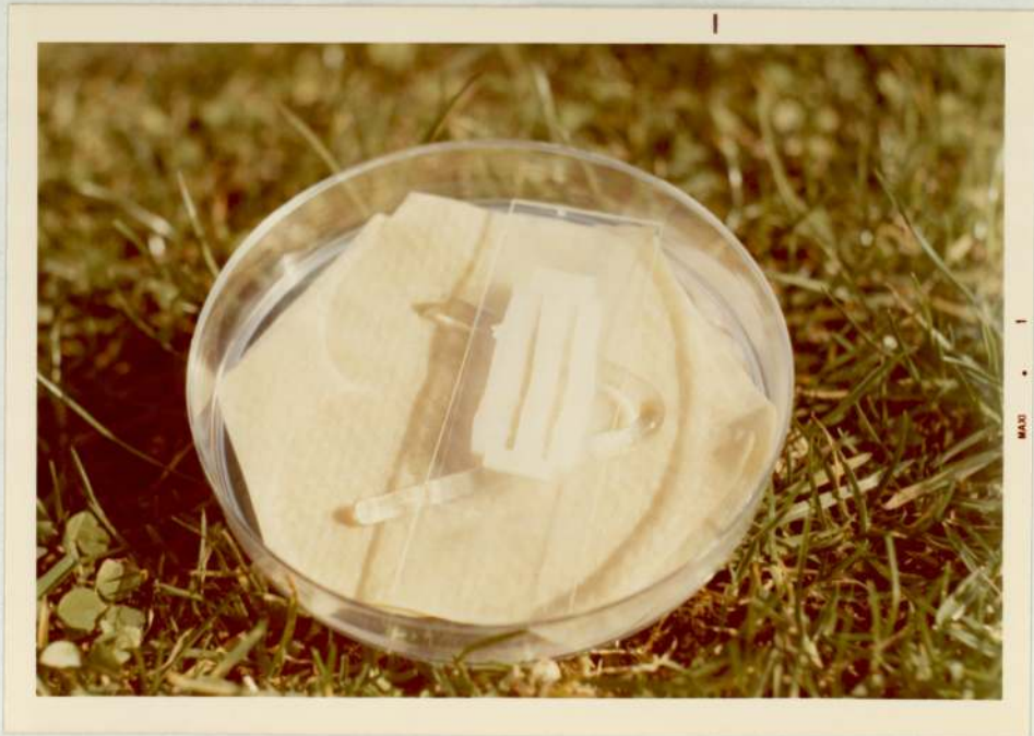
Figure 13. Completed slide culture assembly for microscopic examination of hyphal interaction, with lid removed.
