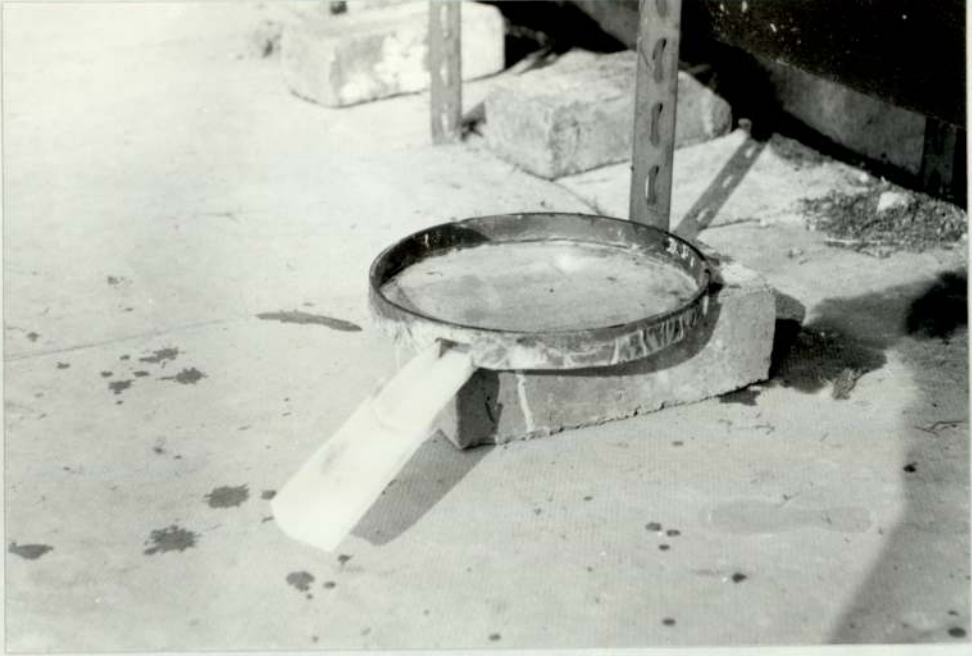
Plate 15. Pilot filter effluent sampling tray
