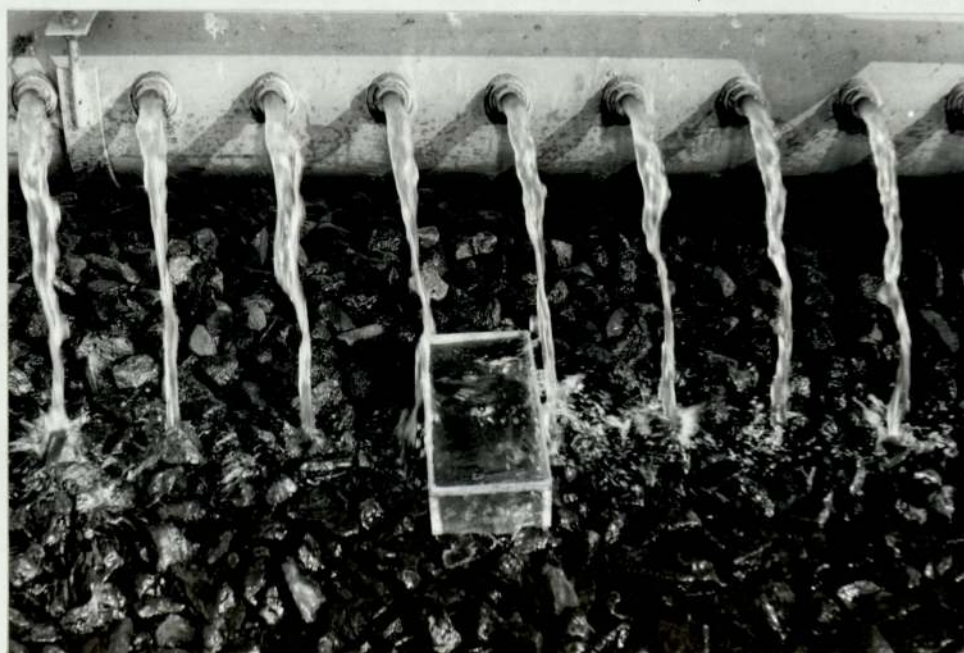
Plate 8. Newly designed fly trap in position on filter
