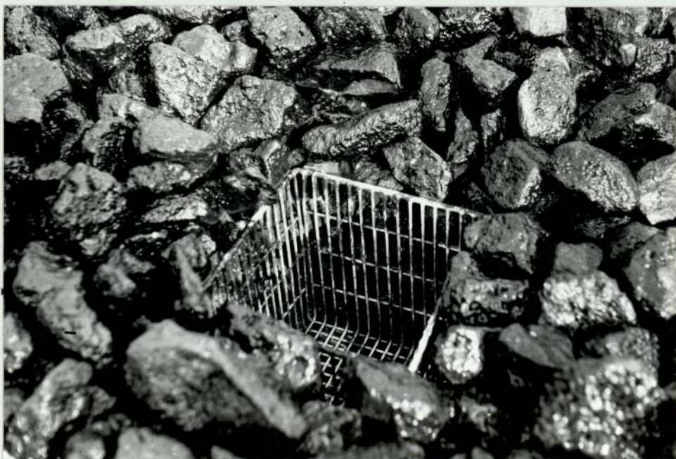
Plate 6. Sample basket in position in filter
