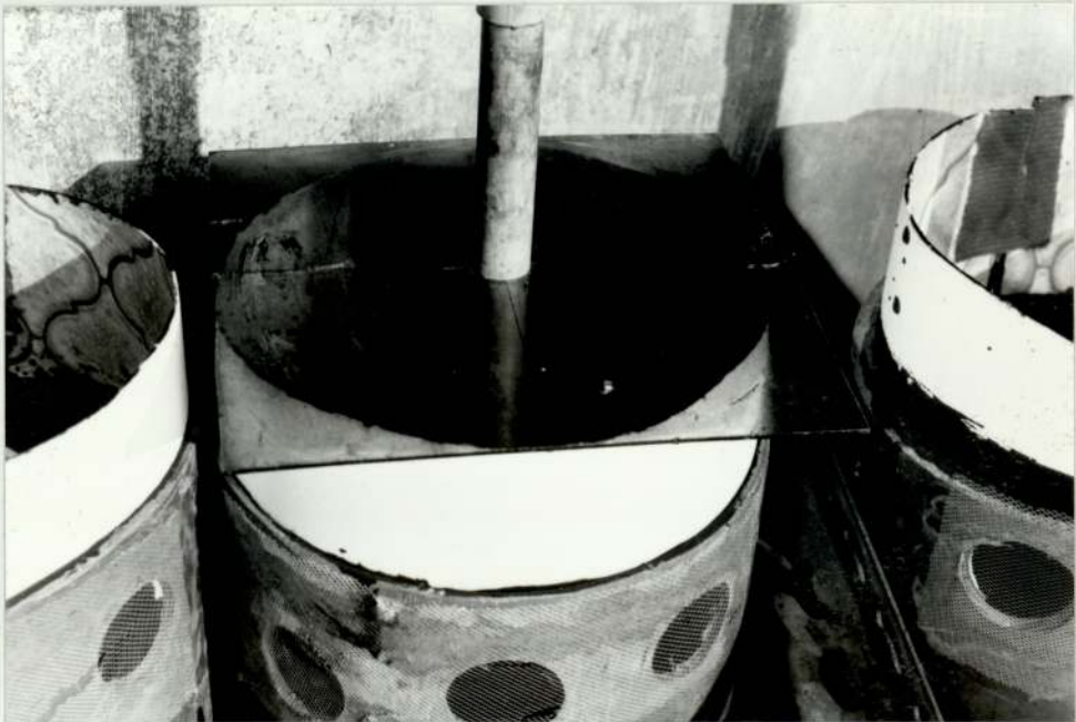
Plate 14. Fly plate in position on pilot filters
