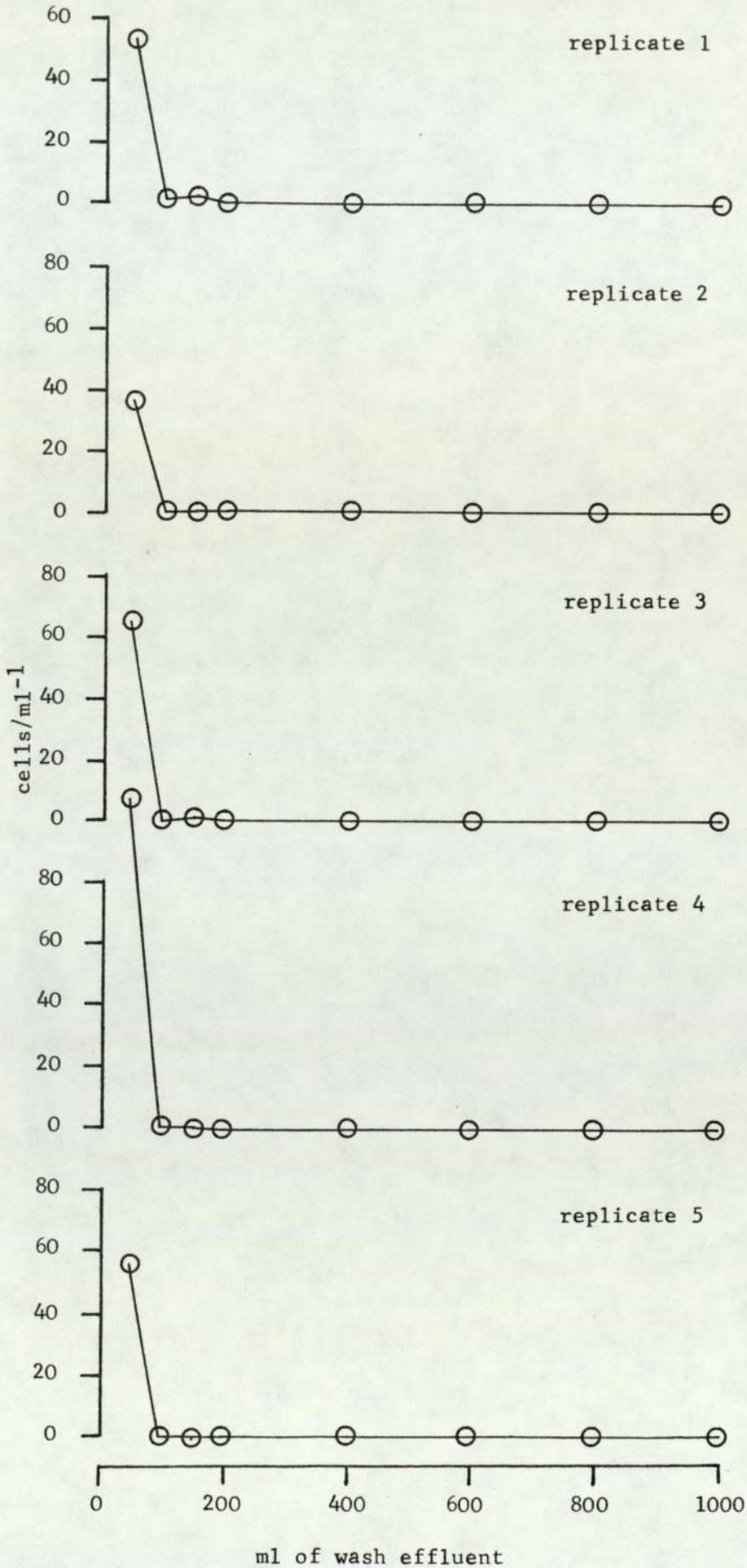
Fig. 7 Removal by rinsing, of unattached bacteria from 5 replicate slides.
