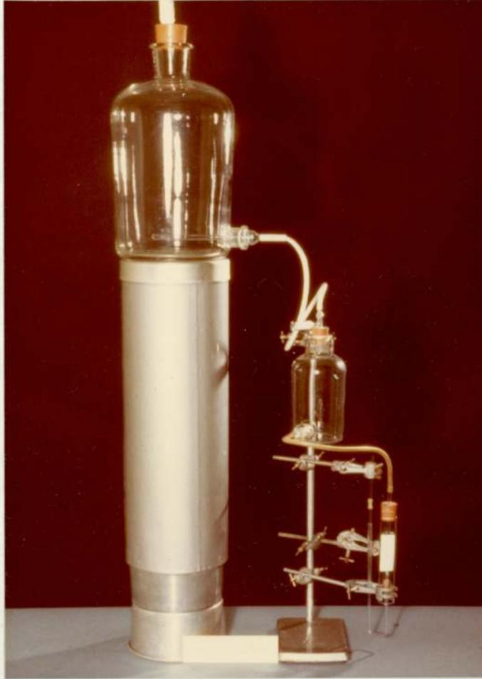
Fig. 3 Assembled sample washing equipment.
