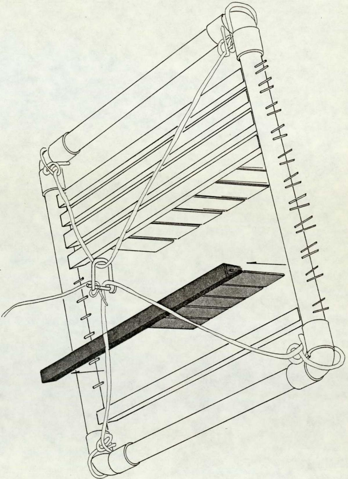
Fig. 2 Short term immersion, ready access sample holder.
