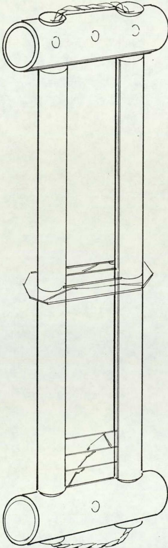
Fig. 1 40 slide sample holder fitted with central stiffener.
