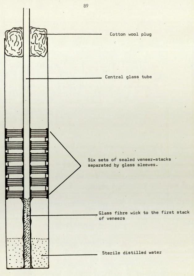
MOISTURE GRADIENT APPARATUS CONTAINING STACKS OF VENEERS
