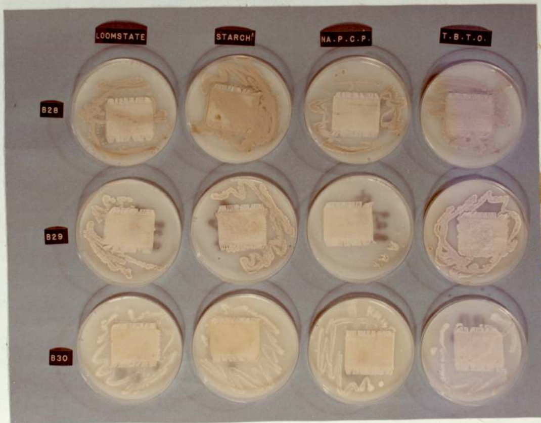
Plate 8. Growth of Streptomyces B28, B29, B30 on loomstate, starch-coated, 0.5%NaP.C.P. & 0.1%T.B.T.O. treated test strips.
