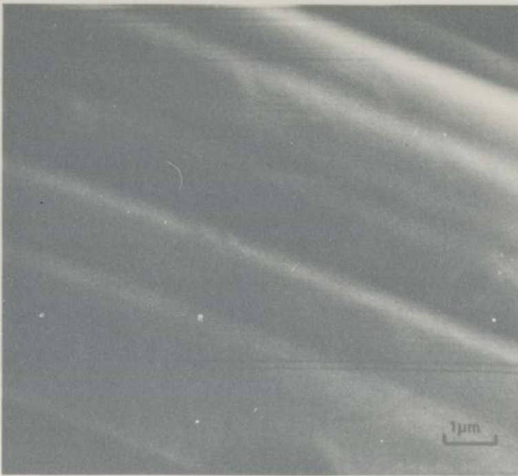
Plate 5.2 A Charcoal Fibre after Reaction with Phenol (x 9750)
