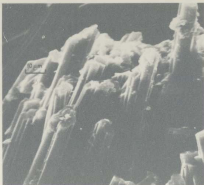
Plate 5.10 Fractured Ends of Charcoal Fibres (x1100)
