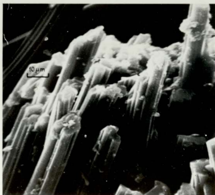
Plate 5.10 Fractured Ends of Charcoal Fibres (x1100)
