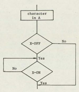
terminal. This 'busy' signal (X-OFF character) can be initiated by the printer if its input buffer is full. On receiving a 'ready' signal (an X-ON character) the H316 exits the waiting loop to proceed with normal program execution. In this way, no information is lost during printing. An example of its use with the H316 Text Editor is shown below.
