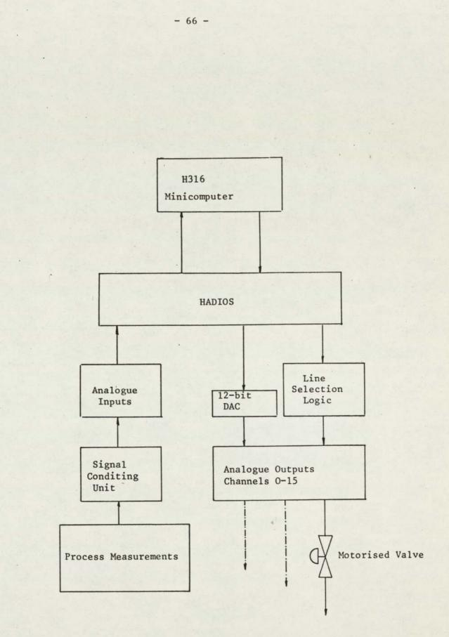
Figure 3.2 A Schematic Diagram of the Computer-Process Hardware Interface
