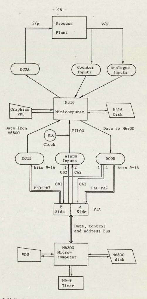
Figure 3.13 Hardware Arrangement for the Linked H316-M6800 Twin Processor
