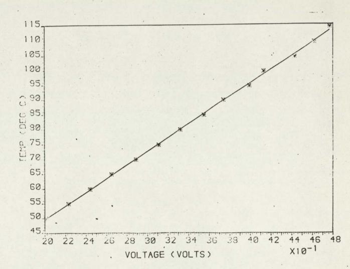
Figure A5.5 Calibration of Topmost tray thermocouple
