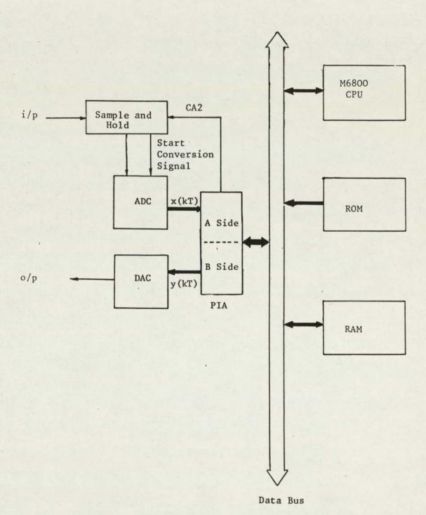
(54) Figure 2.1 Overview of a microprocessor-based digital filter system design
