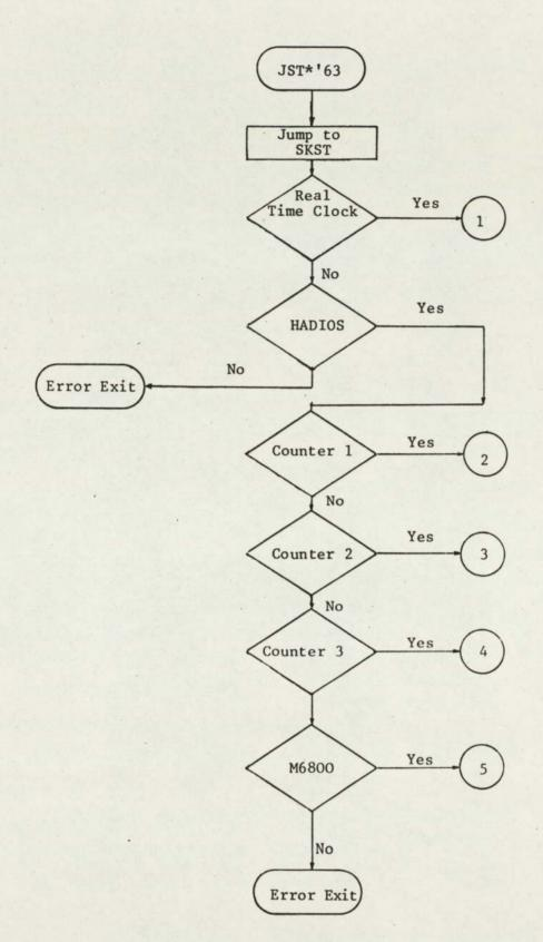
Figure 4.2a Interrupt Source Identification in the H316 Minicomputer
