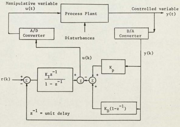
Figure 1.3 Direct Digital Control Loop (P+I+D)
