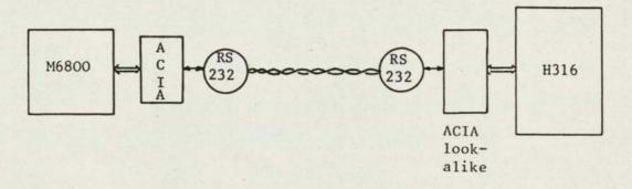
Figure 7.1 A Serial Data Link for the H316-M6800 system: Method 1
