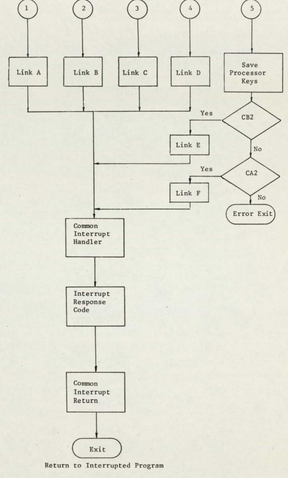
Figure 4.2b Interrupt Handling in the H316 Minicomputer
