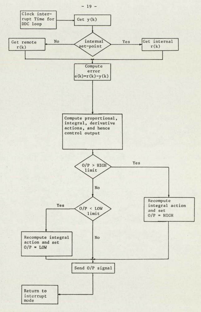
Figure 1.4 Flow Diagram of a Simple Digital PID Controller
