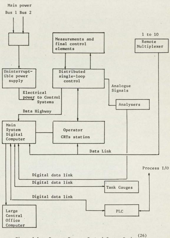
Figure 1.1. Present Process Control System Design.
