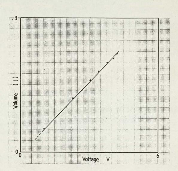
Figure A5.10 Calibration of Reflux Drum Level
