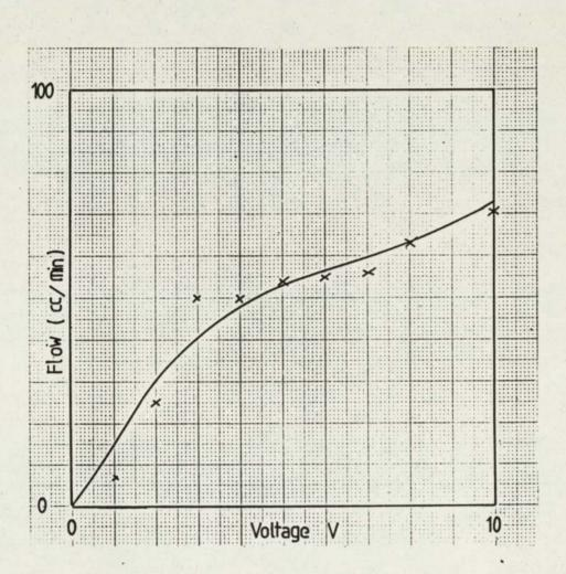
Figure A5.4 Calibration of Distillate Valve, A5
