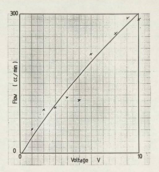
Figure A5.2 Calibration of Bottom product valve, A2
