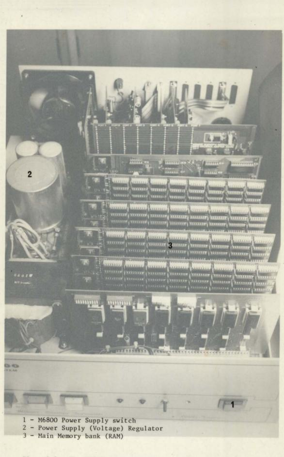
Plate 3.3 The M6800 System Kit (Assembled)
