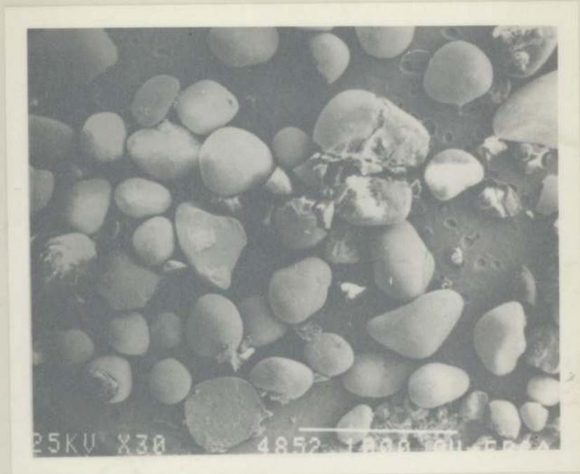
Figure A12.5: Run 51 large crystals fraction sediment
