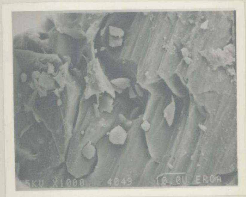
Figure A12.2: Run 33 large crystals fraction sediment
