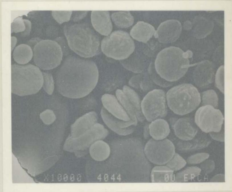
Figure A12.21: Sediment collected from centrifuge tubes after centrifuge tests were carried out on stored product samples
