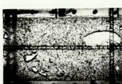
Figure 7.5 Effects of solids size and density on flow regimes and bubble dynamics
