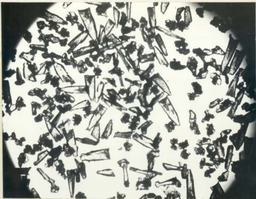
Figure 9.11: Barium chromate crystals grown by the hydrolysis of urea using a mild steel stirring shaft coated with PTFE. epoxy resin.
