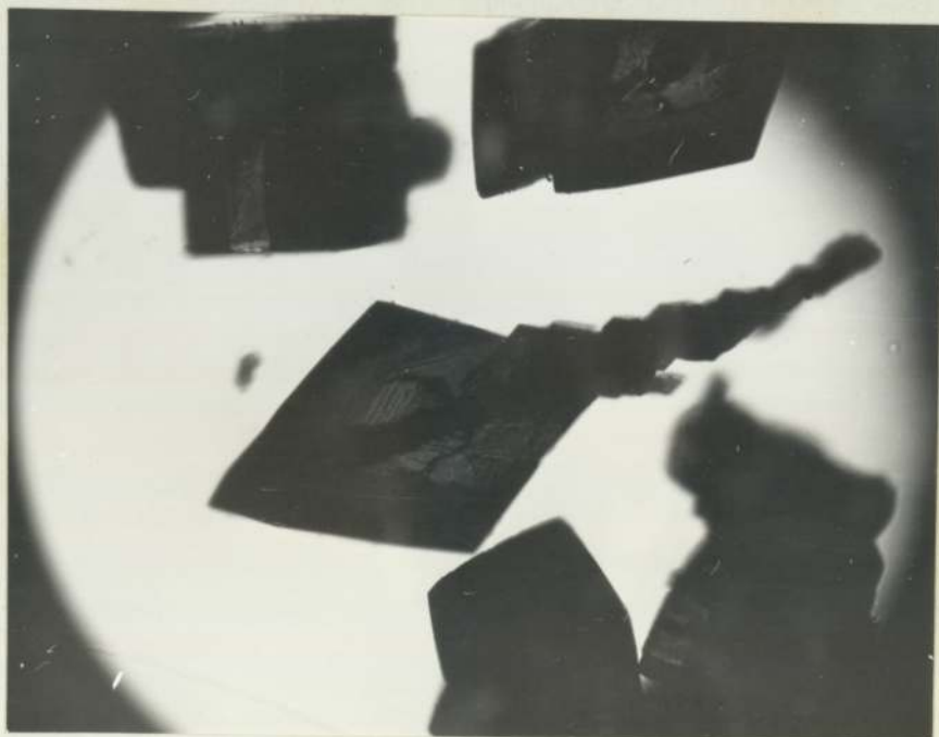
Figure 9.12: Barium chromate crystals grown by the hydrolysis of urea using a mild steel stirring shaft coated with PTFE.
