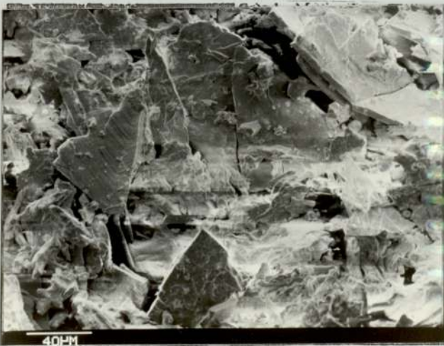
F.6.3. Barium chromate crystals as grown in the presence of Acetic acid.
