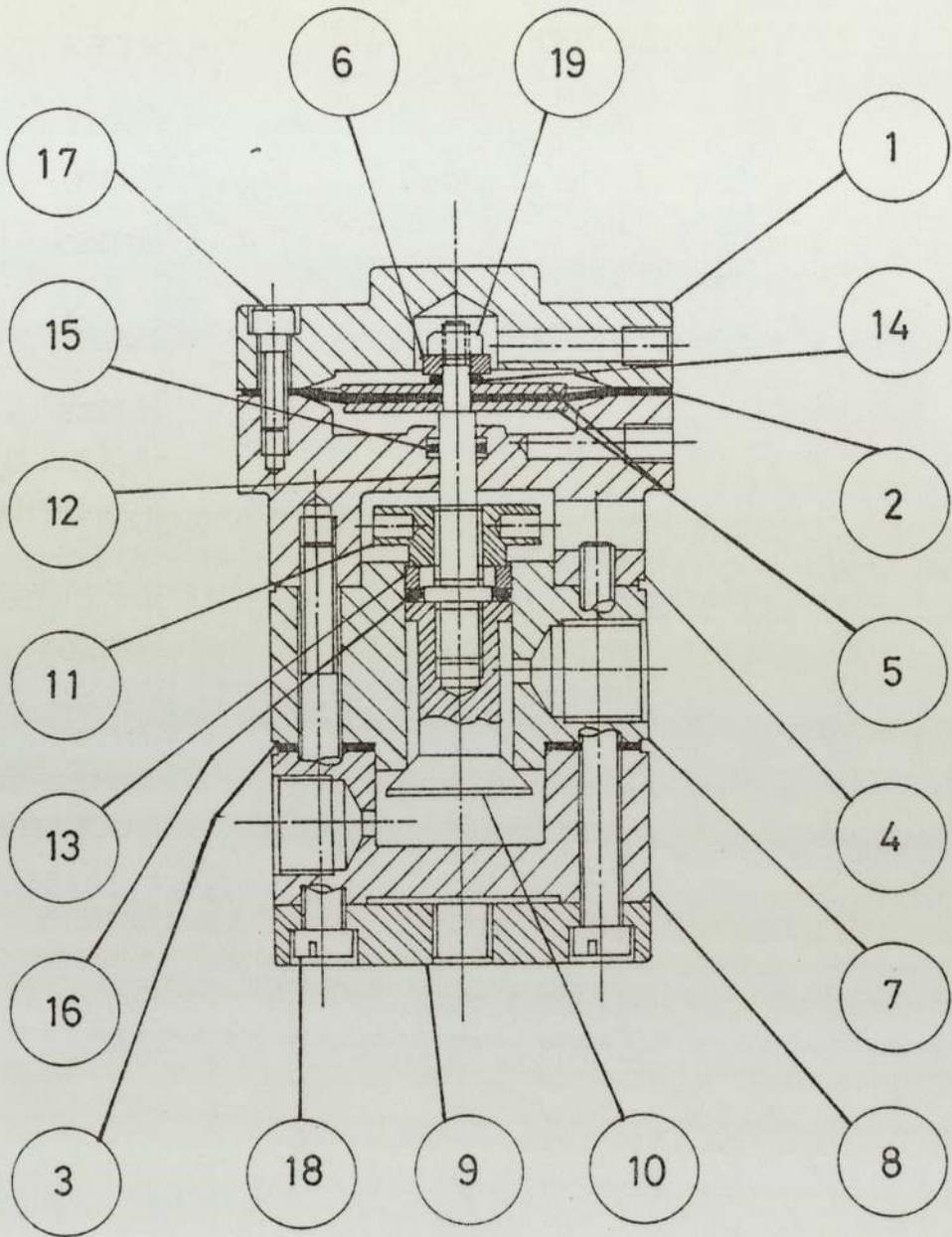
Fig 6.9 Cross-sectional view of pneumatic poppet valve.
