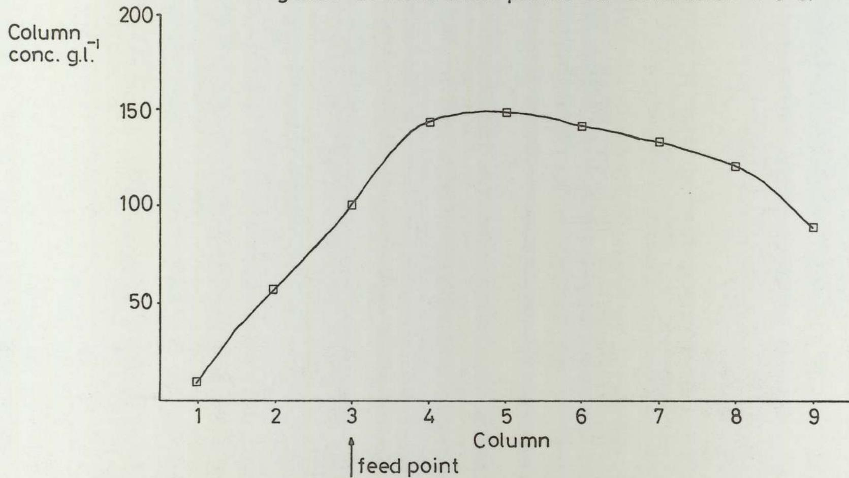
Fig 9.25 Concentration profile for simulation 4-5-4.
