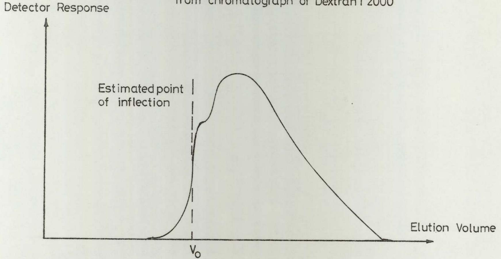
Fig4.5 Elution profile for glucose on Spheron P1000 packed in a 8m.m. i.d. Shandon column.
