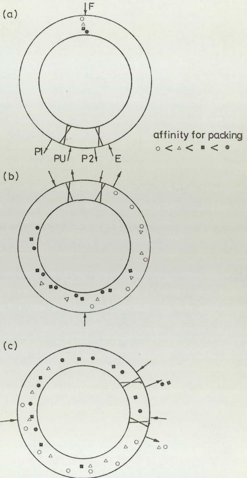
Fig 6.3 Pseudo-steady state distribution for high molecular weight removal.
