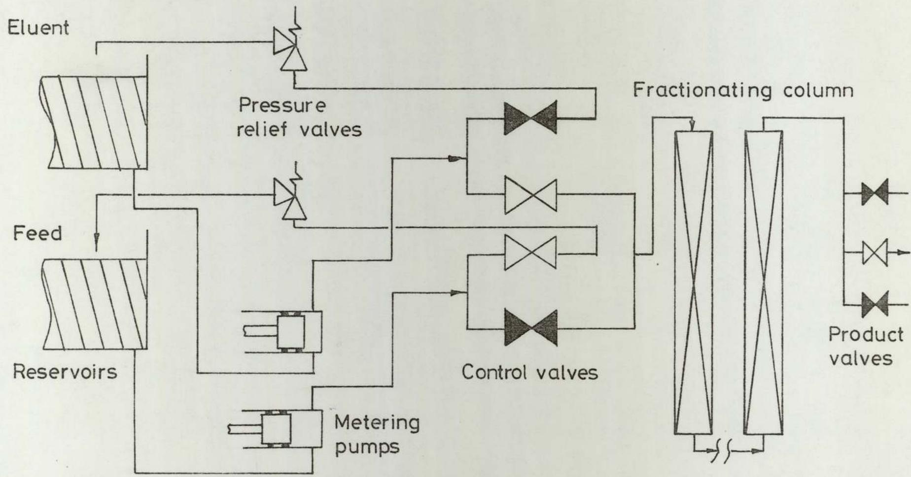
Fig 5.4 Schematic diagram of repetitive batch chromatograph in elution mode
