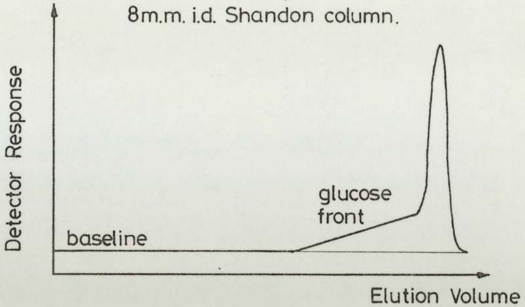
Fig4.6 Elution profile for Dextran plus a glucose marker.
