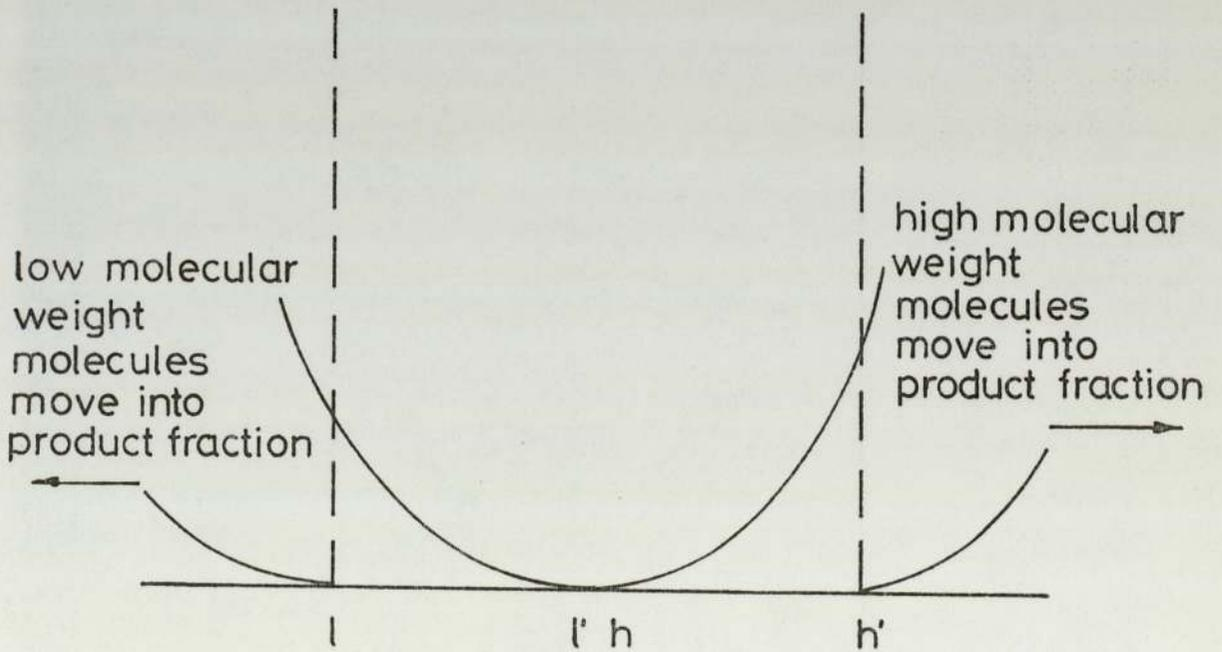
Fig 5.23 Effect of sample volume on elution volume of product fraction.
