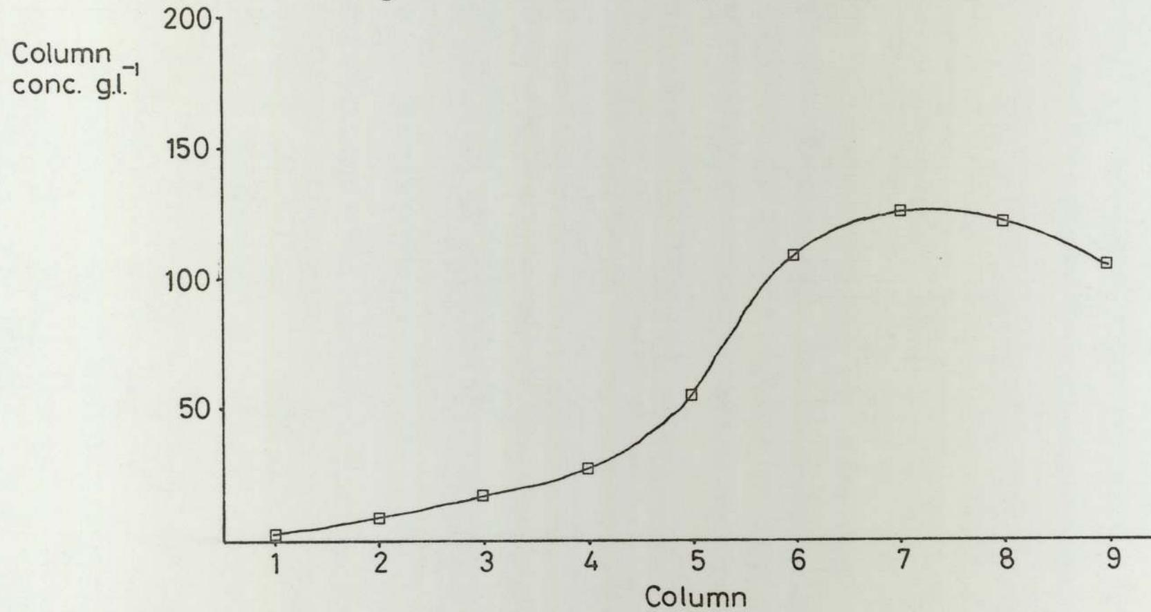
Fig 9.17 Product compositions for simulations with a pre-feed cut-position of 0.7.
