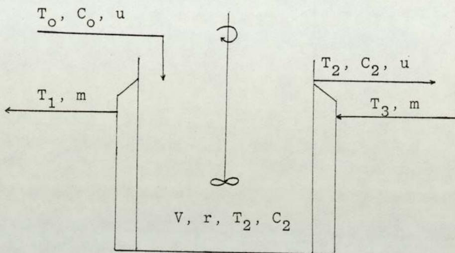
FIG.3.1 A Typical CSTR with a Cooling Jacket
