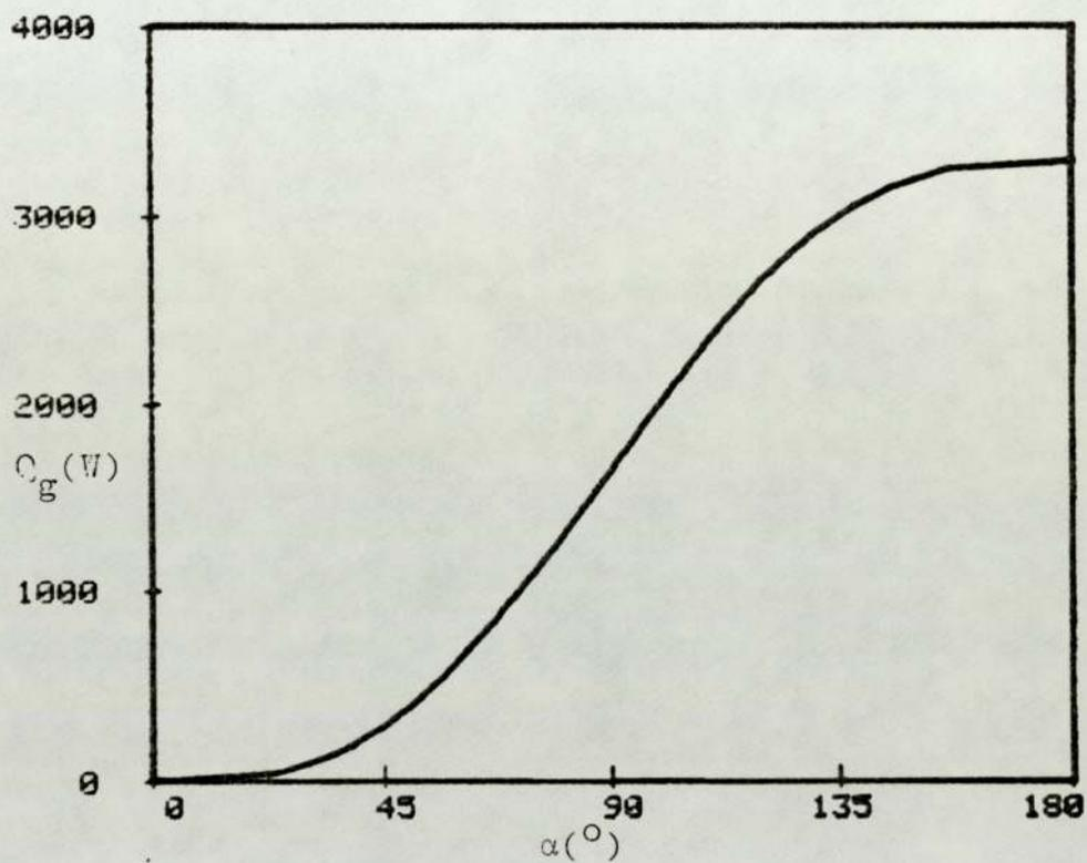
FIG. A.2.1 Heat Output of the Immersion Heaters Versus Trigger Angle
