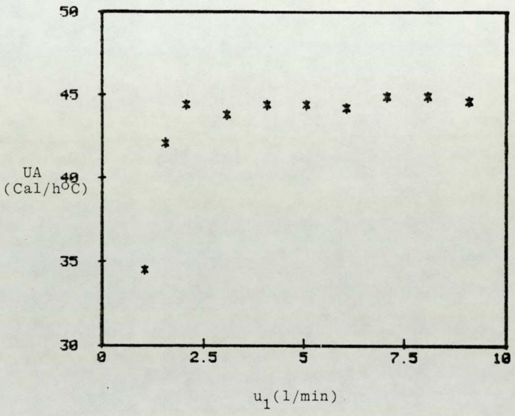
FIG. A.2.5 Heat Transfer Resistance (UA) Versus Jacket Flowrate
