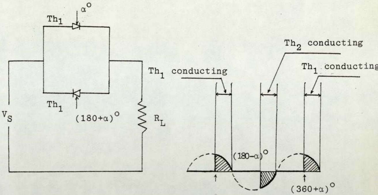
Fig. 4.7 - Circuit and wave forms for inverse-parallel configuration with resistive load
