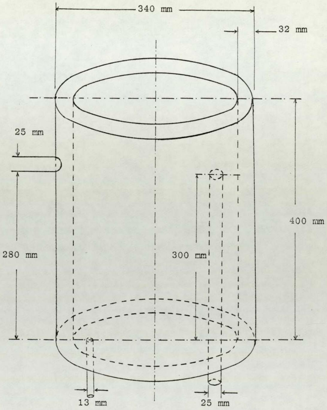
FIG.4.5 The Schematic Diagram of the Jacketed CSTR
