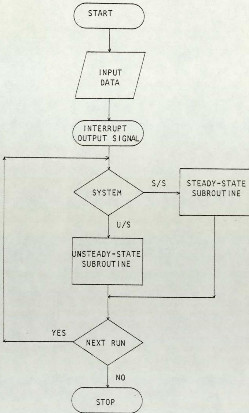
A.4.3 PARTIAL SIMULATION STEADY-STATE COMPUTER FLOW DIAGRAM
