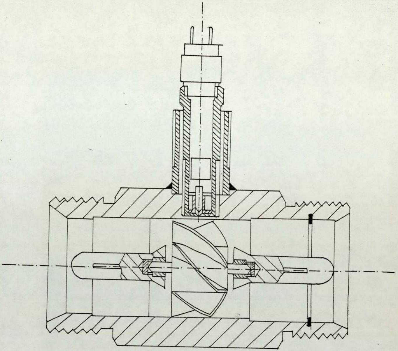
FIG.4.9 Schematic Diagram of the Turbine Flowmeter
