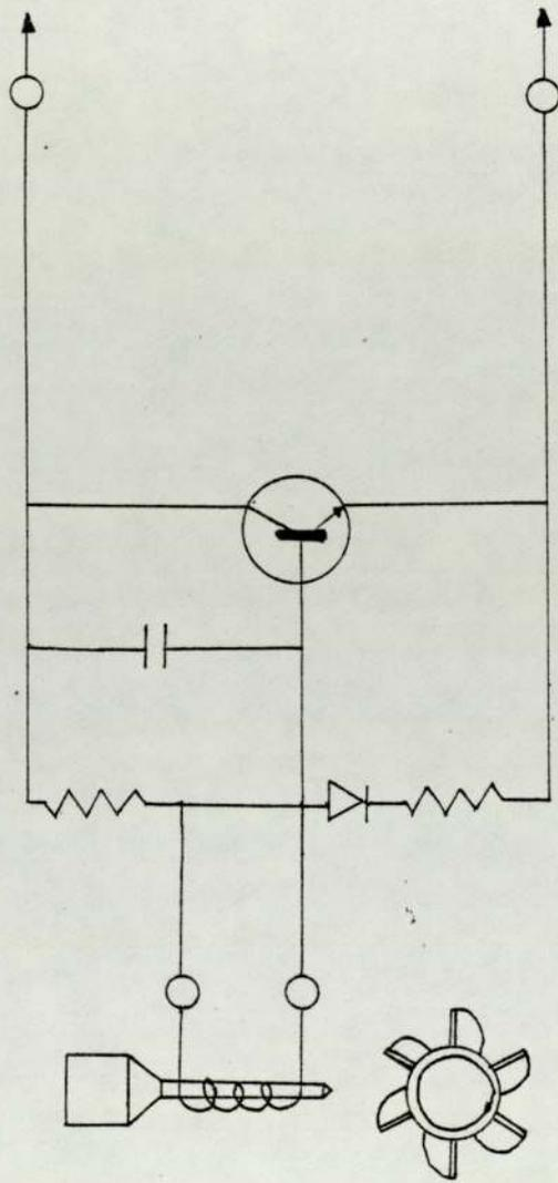
FIG. 4.10 The Magnet, the Coil and the Electrical Circuit of the Turbine Flowmeter
