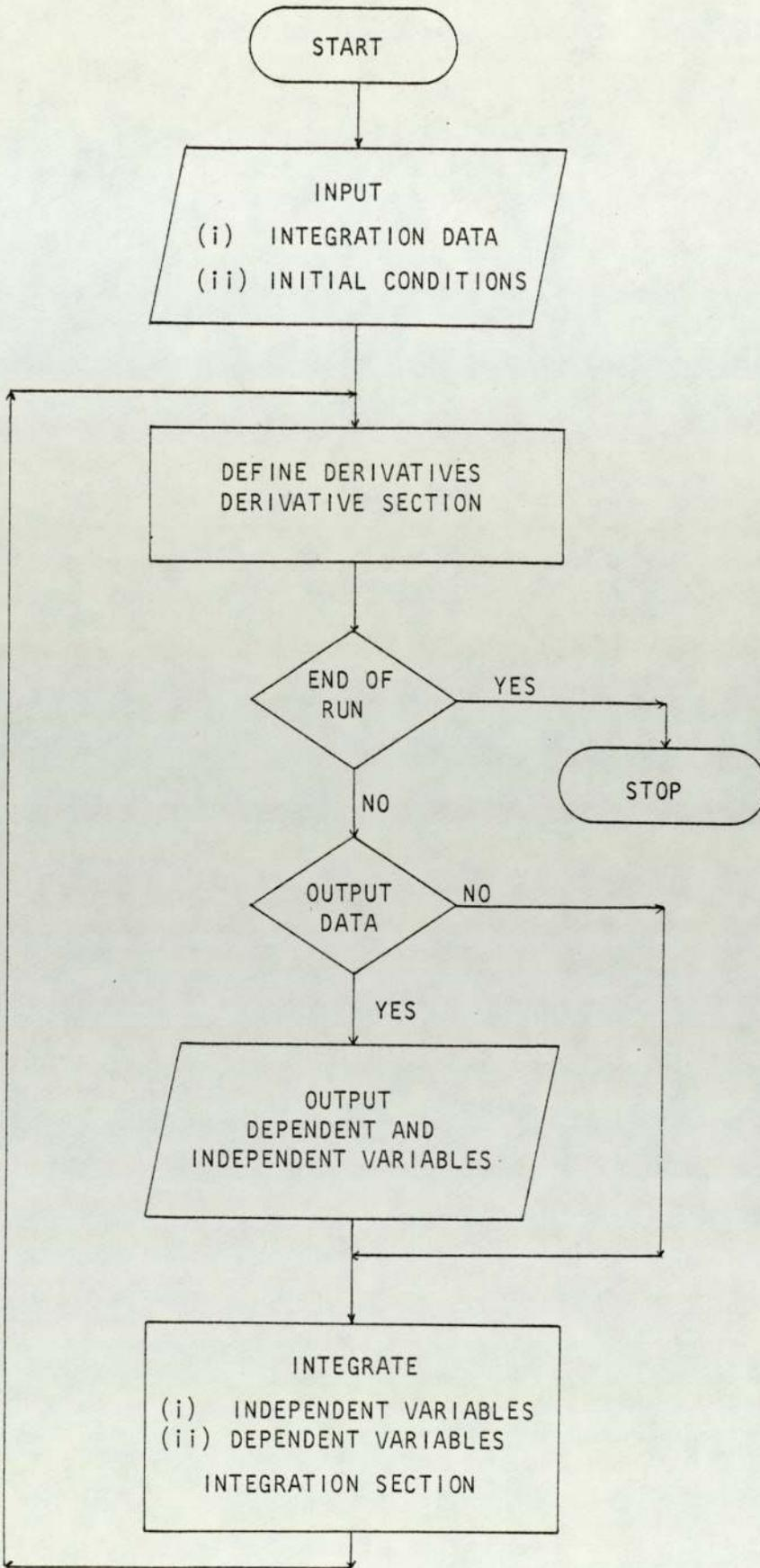
A.4.2 PARTIAL SIMULATION MAIN COMPUTER FLOW DIAGRAM
