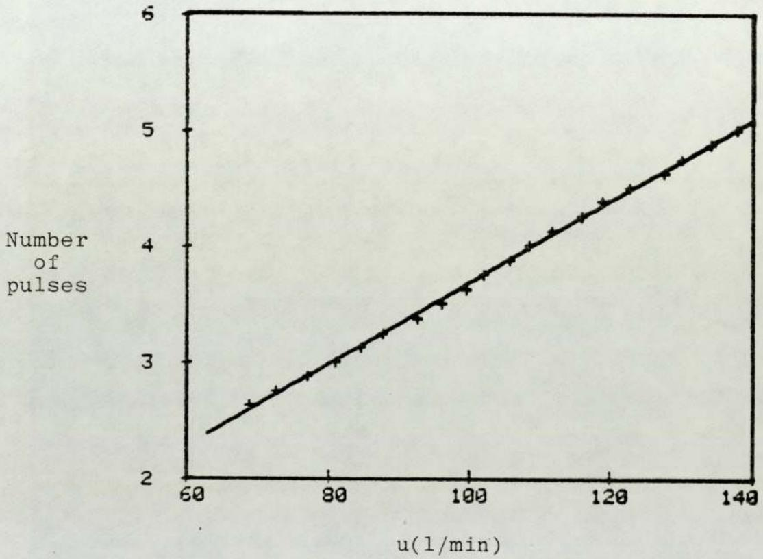
FIG. A.2.4 Number of Turbine Flowmeter Pulses Versus Reactor Throughput
