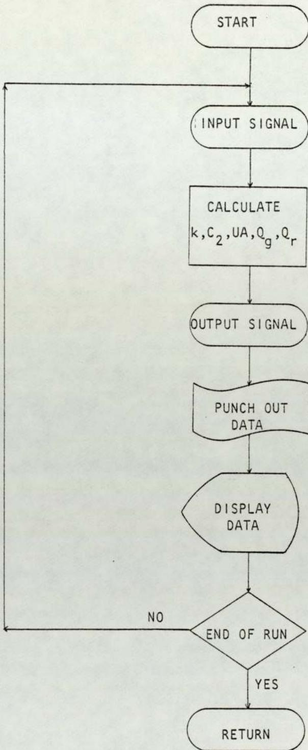
A.4.4 PARTIAL SIMULATION UNSTEADY-STATE COMPUTER FLOW DIAGRAM
