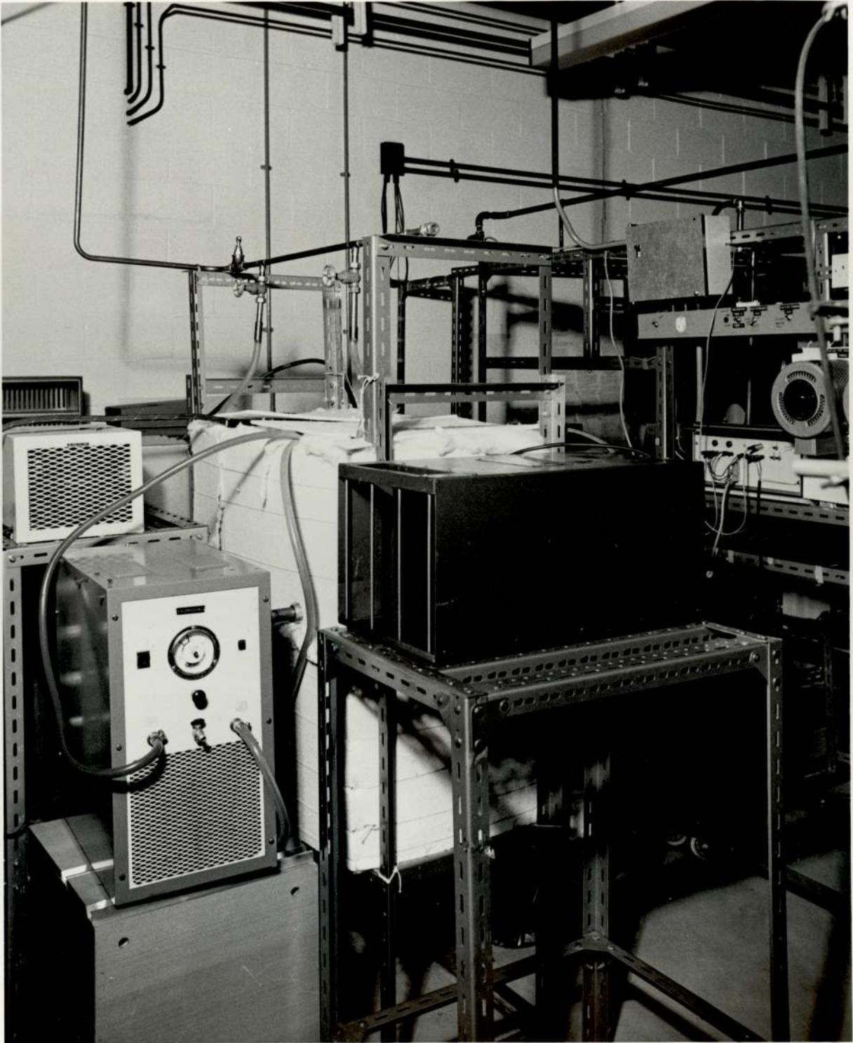
FIG. 4.4 The Jacket CSTR used in the Project
