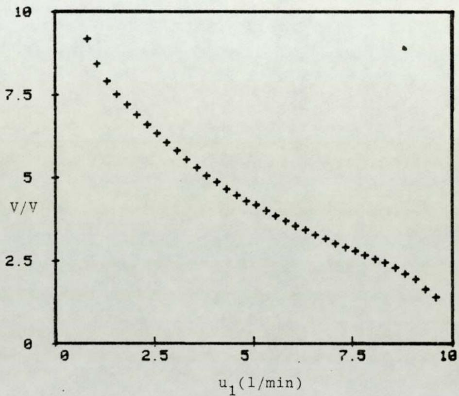
FIG. A.2.3 Analogue Output Voltage Versus Jacket Flowrate with Equal Interval
