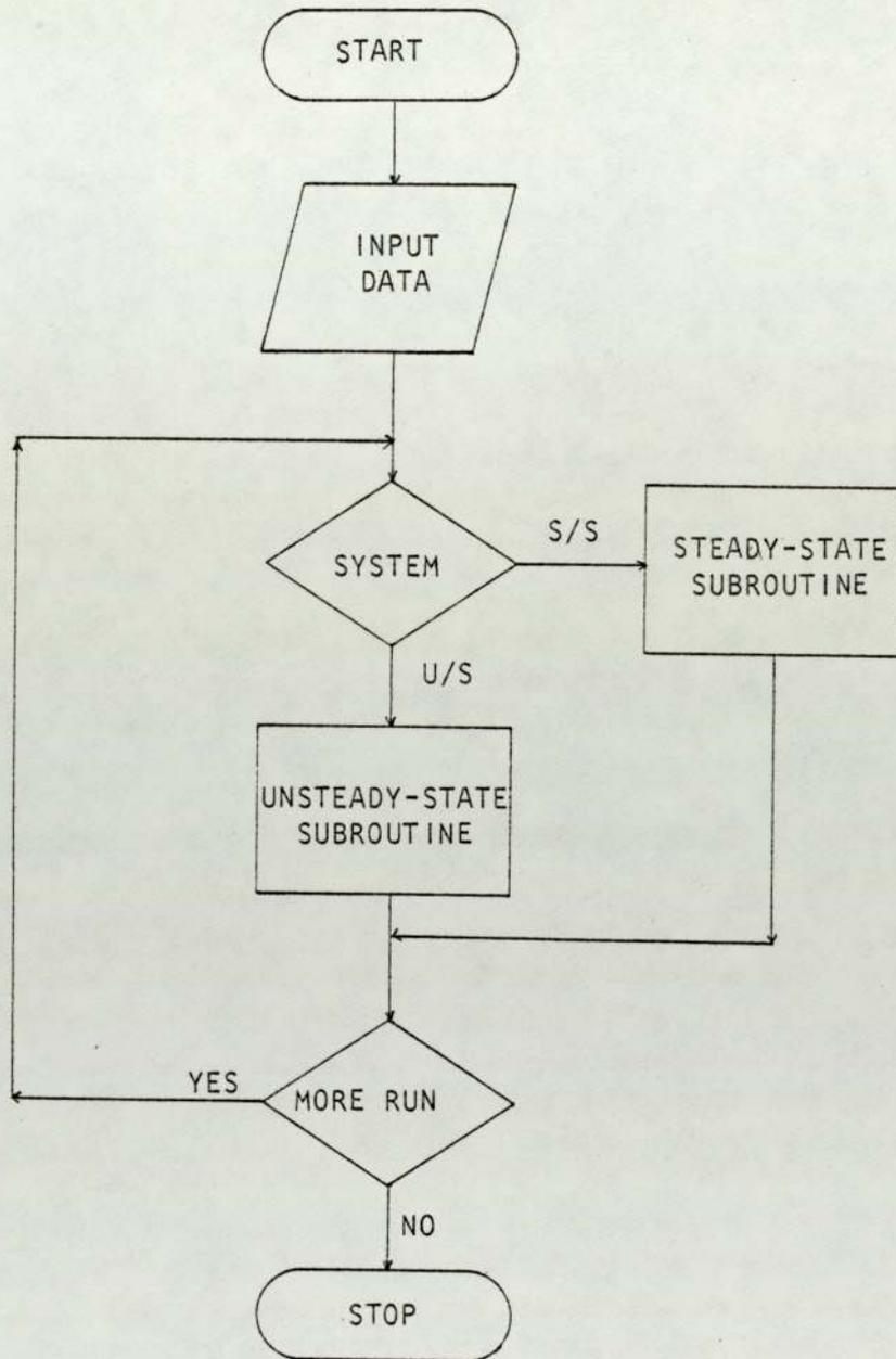
A.4.6 TOTAL SIMULATION STEADY-STATE COMPUTER FLOW DIAGRAM
