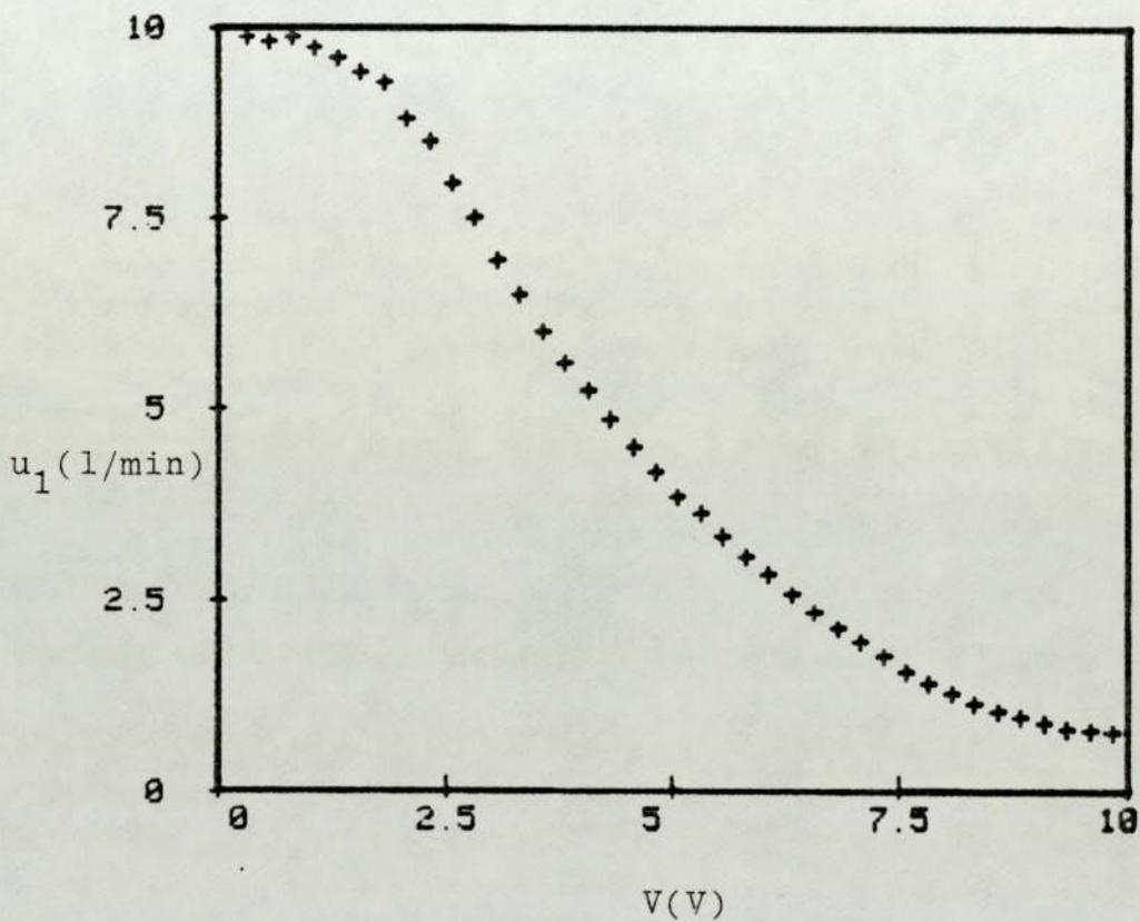
FIG. A.2.2 Jacket Flowrate versus Analogue Output Voltage with Equal Interval
