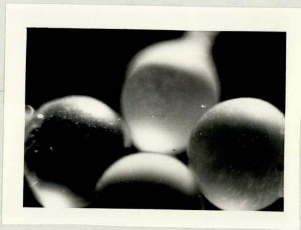
Four glass beads; ratio of high to low surface energy varied by coating with p. t. f. e. aerosol (e. g. in this example three glass beads were coated to give a ratio of 1:3 and a cubical aperture).
