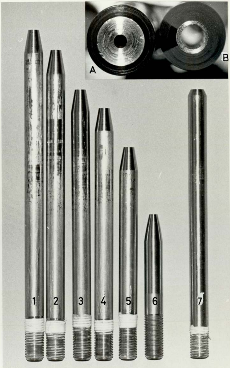
FIGURES 3,10 : VIEW OF THE NOZZLE(7) WITH THE FULL RANGE OF RECEIVERS USED (1-6).
