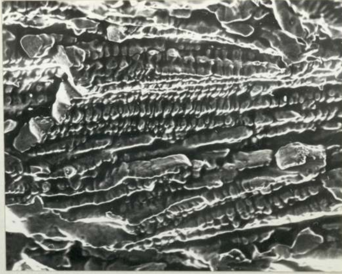
Fig 47. Crack surface showing dendrites with broken ends, MC11 (0.080% S, CSF = 9). X 500
