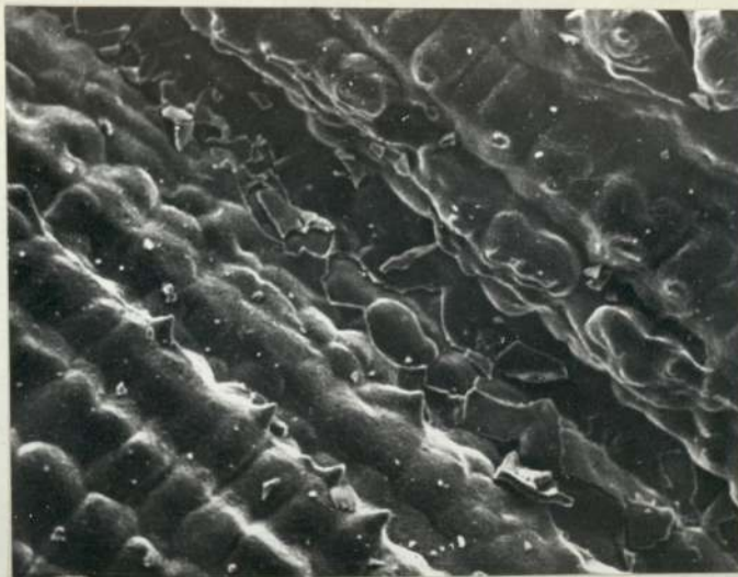
Fig 37. Oxidized crack surface with a general dendritic pattern, MA 7 (SAE4130, 0.032% S, CSF = 62). X 500
