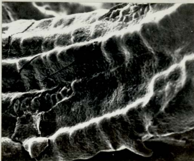
Fig 36. Oxidized solidification crack surface, the true solidification structure being obscured by the presence of oxide skins. MD18 (EN5, 0.030% S, CSF = 68). X 600
