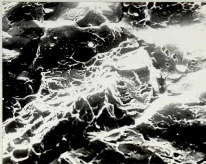
Fig 34. Extended fracture surface of solidification crack caused by mechanical rupturing at room temperature for a less crack susceptible steel weld. MA5 (SAE4130, 0.007% S, CSF = 1).
