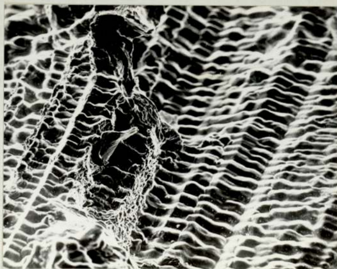
Fig 52. Crack surface showing some area being in a mushy state during solidification cracking, MB6 (SAE4130, 0.40% C, 0.012% S, CSF = 31). X 1000
