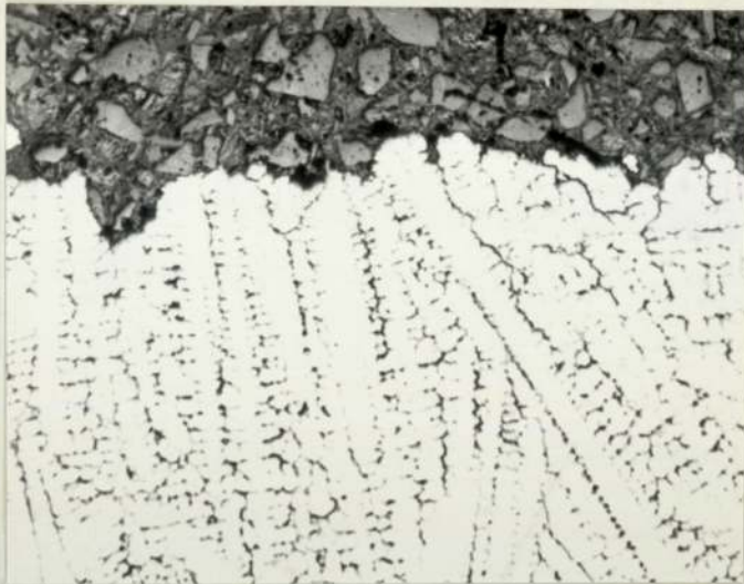
Fig 25. Flat section of the weld of MA3 (SAE4130, 0.042% S, 0.005% P, CSF = 62) showing the dendrites near a centreline crack boundary. Specimen etched in a solution of saturated picric acid with a wetting agent. X70.
