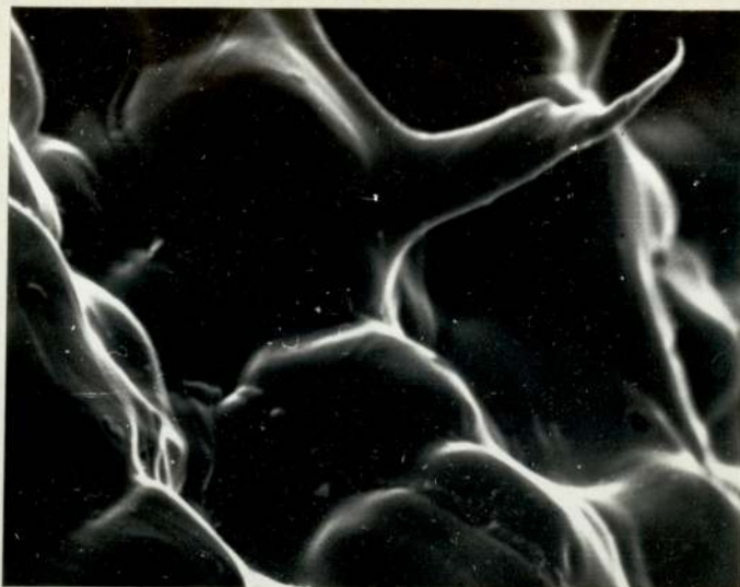
Fig 45. Crack surface showing extended tips of necked down bridges between grains, seen in the weld of MA7 (SAE4130, 0.032% S, 0.17% Mn, CSF = 62). X 3000
