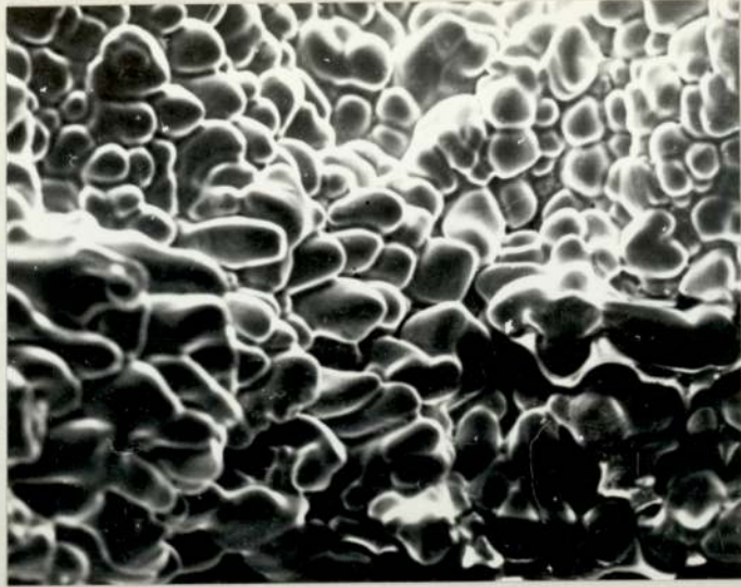
Fig 39. Gas pore interior with round dendritic tips or equiaxed grains, MA7 (SAE4130, 0.032% S, CSF = 62). X 1000
