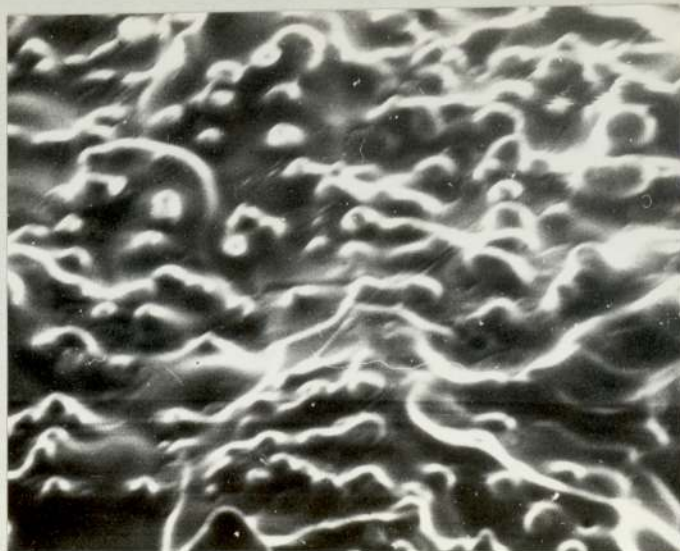
Fig 42. Stereomicrograph of solidification crack surface with globules, MC12 (0.170% S, 0.016% O, CSF = 63).
