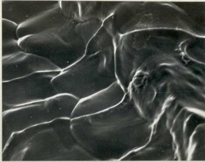
Fig 53. Crack surface with ridges seen in the specimen of a less crack susceptible steel, MA2 (SAE4130, 0.009% S, CSF = 12). X 1000
