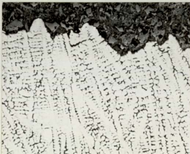
Fig 26. Flat section of the weld of MA3 (SAE4130, 0.042% S, 0.005% P, CSF = 62) showing the dendrites near a centreline crack boundary. X70.
