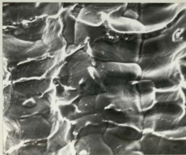
Fig 54. Crack surface with ridges seen in the specimen of a less crack susceptible steel. The ridges contain more sulphur than the matrix does. Weld of MA2 (SAE4130, 0.009% S, CSF = 12). X 800
