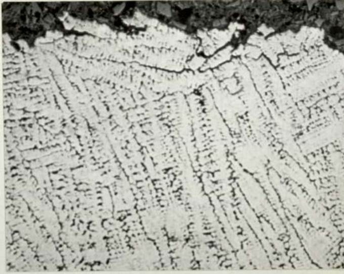
Fig 27. Flat section of the weld of MD19 (EN19, 0.015% S, 0.042% P, CSF = 53) showing the detachment and rupture of dendrites near the crack boundary. X70.
