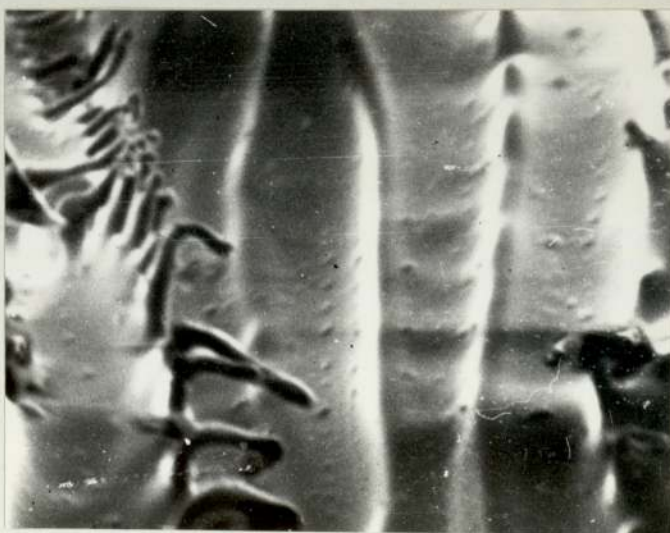
Fig 46. Crack surface with a series of necked down bridges, seen in the weld of MC12 (Fe-Mn-S-O alloy, 0.17% S, 0.016% O, 0.03% Mn, CSF = 63). X 2000
