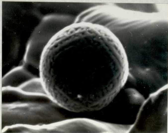
Fig 55b. Freely solidified ball on the crack surface of MA7 weld (SAE4130, 0.28% C, 0.032% S, CSF = 62). The ball diameter is about 20 \mu\text{m} . X 5000
