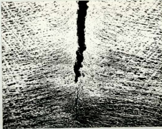
Fig 31. A stereomicrograph of a weld surface of MA3 (SAE4130, 0.042% S, 0.006% P, CSF = 62) with centre-line cracks, slightly etched. X 20
