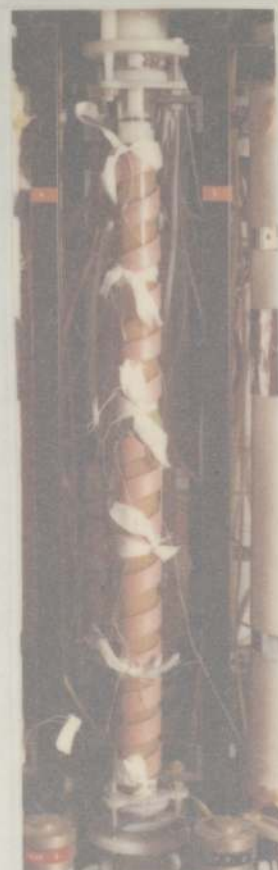
(c) Heating Tape System
