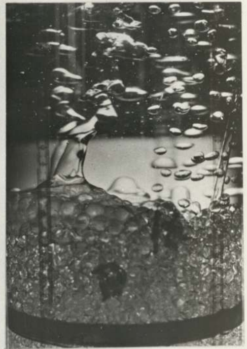
(D) Half Wetted - Half Non-Wetted Illustrating Jetting and Secondary Droplet Formation
