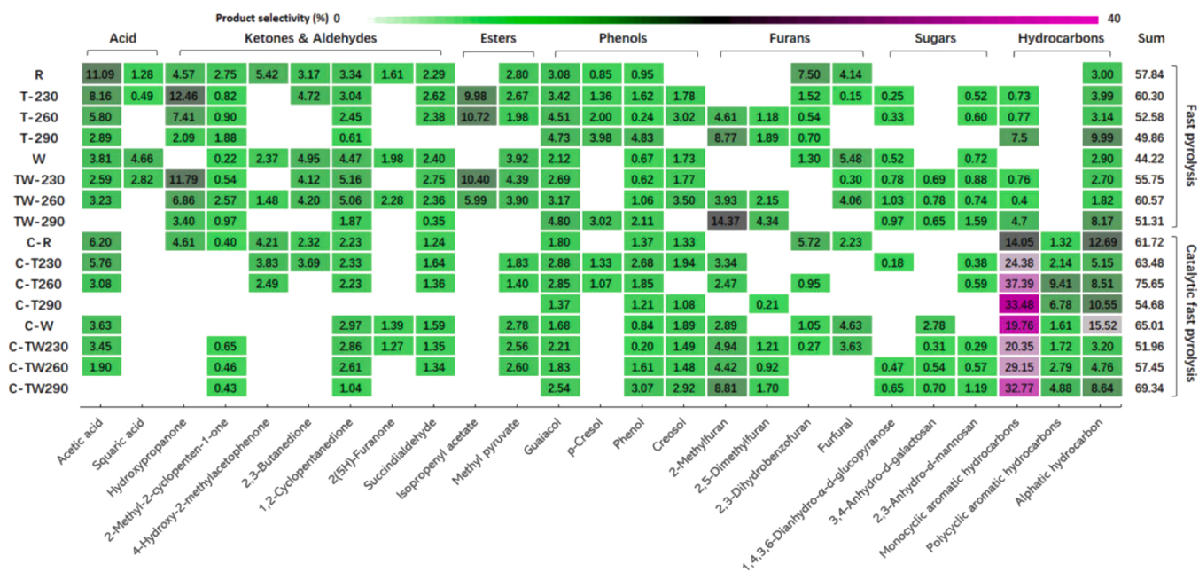
Fig. 3. Products selectivity for liquid component products. The sample name indicates Raw material (R), Torrefaction (T), Acid washing (W), and catalytic process (C). The numbers refer to torrefaction temperatures.
