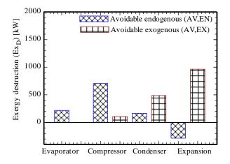
Fig. 4. Advance exergy analysis for NH<sub>3</sub> in all components.
