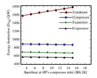
Fig. 5. Effect of SH on the HP system.
