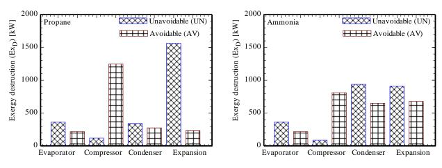
*Fig.* 3(*a*). Avoidable and unavoidable exergy destruction in all components for propane.
