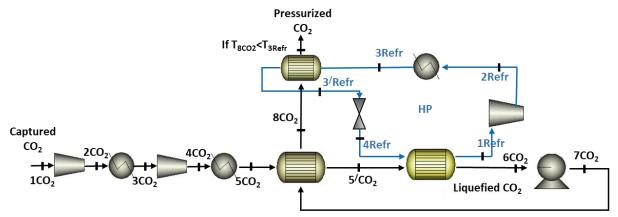
Fig. 6. Improved HP design for CO<sub>2</sub> liquefaction.
