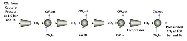
Fig. 1. Benchmark case for CO<sub>2</sub> pressurization.
