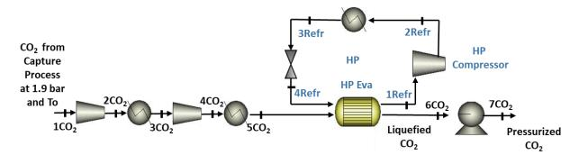
Fig. 2. Proposed design for CO<sub>2</sub> pressurization.
