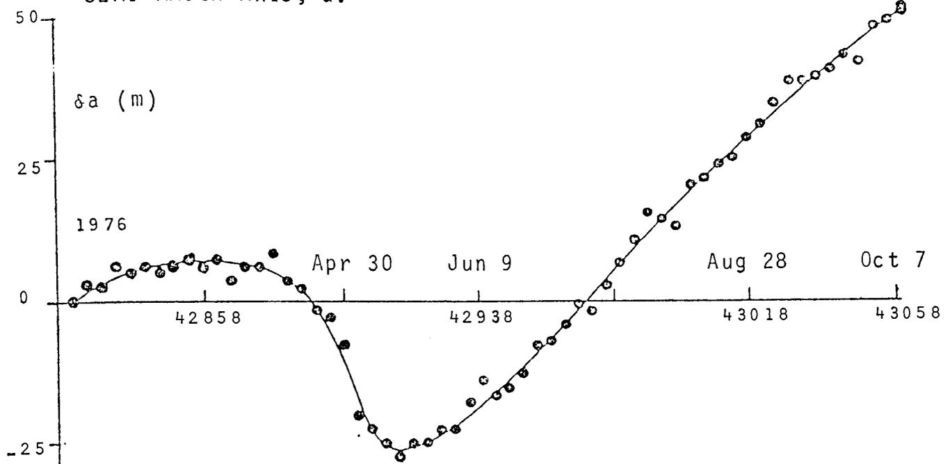
Fig. 28. THE EFFECTS OF EARTH REFLECTED RADIATION ON THE ECCENTRICITY, e.
