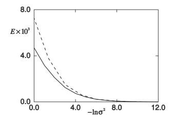
Figure 3: A plot of training error versus  $-\ln \sigma^2$  (dashed curve) for training with noise having input variance  $\sigma^2$ . Also shown on the same scale is the corresponding plot of training error versus  $-\ln \nu$  (solid curve) for the regularized error function given by given by (22) and noise-free data. The data set was taken from a problem concerned with the monitoring of oil flows along multi-phase pipelines [4].
