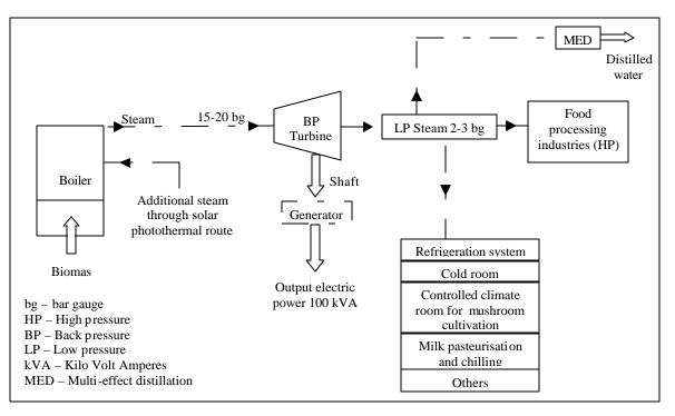
Fig. 1- System based on boiler route
