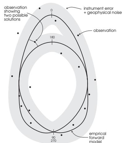
**Figure 2:** A theoretical sketch of the relationship between backscattered radiation and wind direction, for a fixed wind speed. This corresponds to a slice across the ‘cone-like’ manifold. The height up the cone defines the wind speed.
