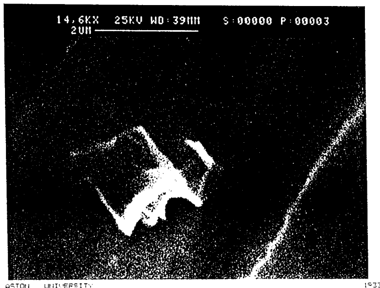
Figure 5.2 Scanning electron micrograph of a montmorillonite platelet
